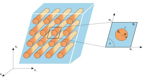
Figure 1. Composite with rhombic array of circular cylinders embedded into a matrix and the unit cell.
