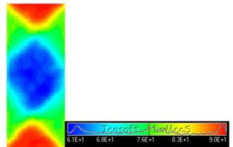
**Fig 6** Shear angle in a plain weave fabric bias-extension test obtained from DIC [25]. (The angles given on the scales are 90°-  $\gamma$ )
