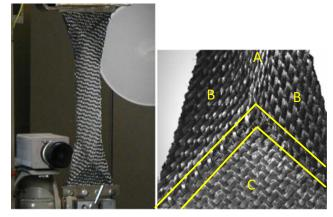
Fig. 27 Transition layer between the zones with constant shear in a biasextension test
