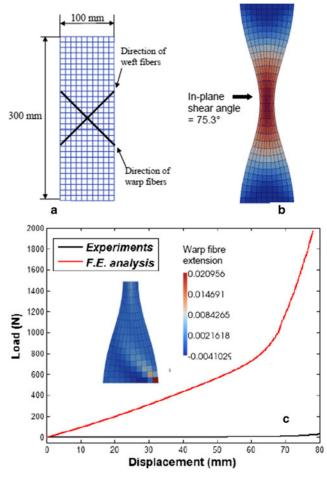
Fig. 24 (a) Initial mesh aligned with the specimen. The fibers are oriented at  $\pm 45^{\circ}$  (b) Deformed mesh for a 65 mm displacement (c) Load on the tensile machine obtained by simulation and by experiments and fibre extensions [72]
