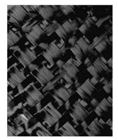
Fig. 29 Unbalanced fabric
