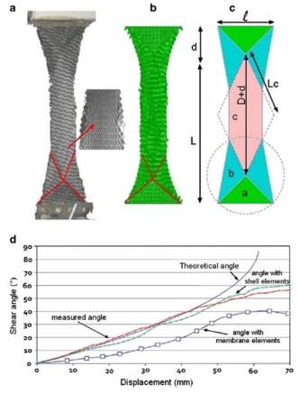
Fig. 33 Bias-extension test for 58° shear angle with local sliding (a) experiments, (b) corresponding mesoscopic finite element simulation. (c) pin-joint kinematics (d) Shear angle as a function of displacement, including theory (Eq. (1)), experimental test, and simulations with shell and membrane elements [90]
