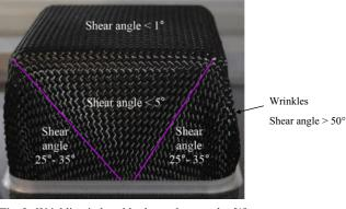
Fig. 2 Wrinkling induced by large shear angles [1]
