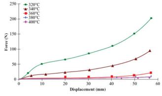
Fig. 15 Bias-extension test load in function of the temperature [52]
