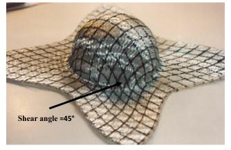
Fig. 1 Forming a woven reinforcement on a double curve shape requires in-plane shear deformations
