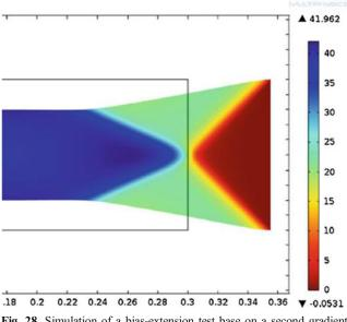
Fig. 28 Simulation of a bias-extension test base on a second gradient theory. Transition layers for the shear angle. [76]
