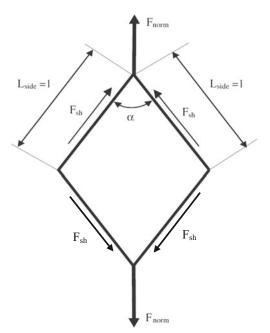
Fig. 8 Normalized load and shear load on a rhomboid with unit side
