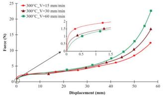
Fig. 17 Load versus displacement curves for carbon/PPS prepreg at 300 °C for different displacement rates [51]
