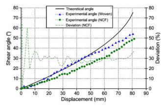
**Fig. 22** Bias-extension test on a NCF. Comparison between theoretical and experimental shear angle versus displacement of the grip. Angle deviation from theoretical angle (dashed line) [63]
