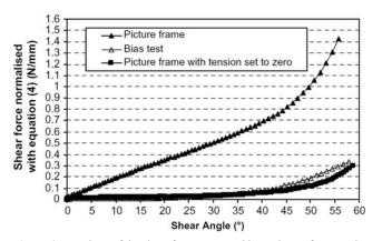
Fig. 5 Comparison of the shear force measured by a picture-frame and a bias-extension test [33]
