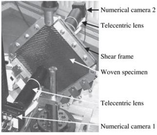
Fig. 3 Picture frame equipped with an optical system
