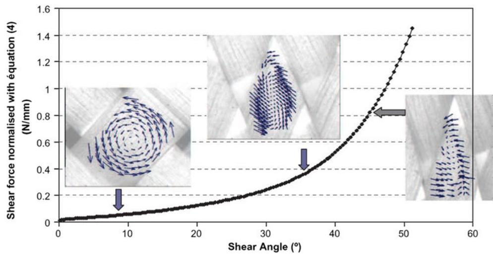
yarns. Then the geometry of the woven cell leads to yarns lateral contacts. The yarn is transversely compacted and this compaction is more important as the shear increases. It can lead to off-plane wrinkling.
