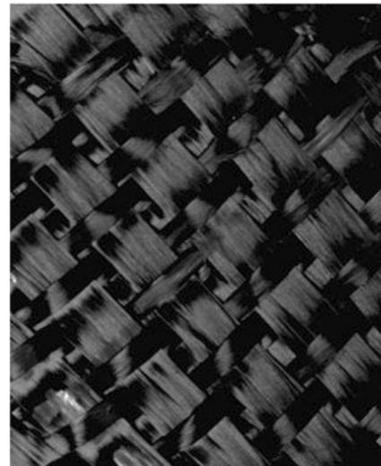
**Fig. 29** Unbalanced fabric
