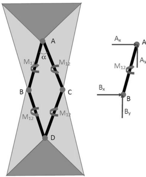
Fig. 10 Static analysis of the bias-extension test
