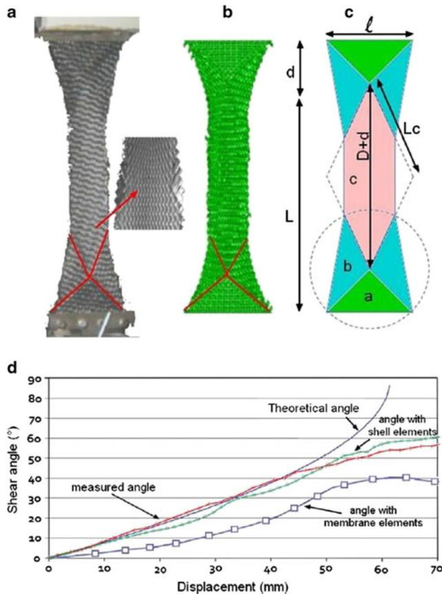
**Fig. 33** Bias-extension test for  $58^\circ$  shear angle with local sliding (a) experiments, (b) corresponding mesoscopic finite element simulation. (c) pin-joint kinematics (d) Shear angle as a function of displacement, including theory (Eq. (1)), experimental test, and simulations with shell and membrane elements [90]
