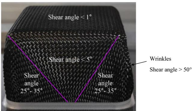
**Fig. 2** Wrinkling induced by large shear angles [1]
