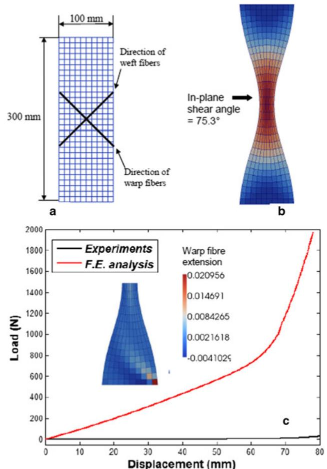
**Fig. 24** (a) Initial mesh aligned with the specimen. The fibers are oriented at  $\pm 45^\circ$  (b) Deformed mesh for a 65 mm displacement (c) Load on the tensile machine obtained by simulation and by experiments and fibre extensions [72]
