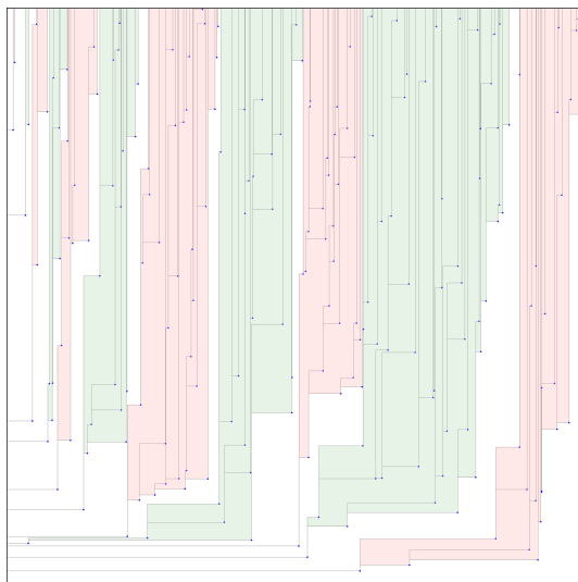
Figure 1: Sorting a random permutation of size n=200 into binary heaps. Here, 11 trees coloured alternatively in red and green are required.
