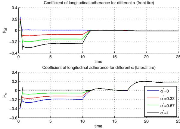
Fig. 8. Front and rear longitudinal adhesion for different values of  $\alpha^*$
