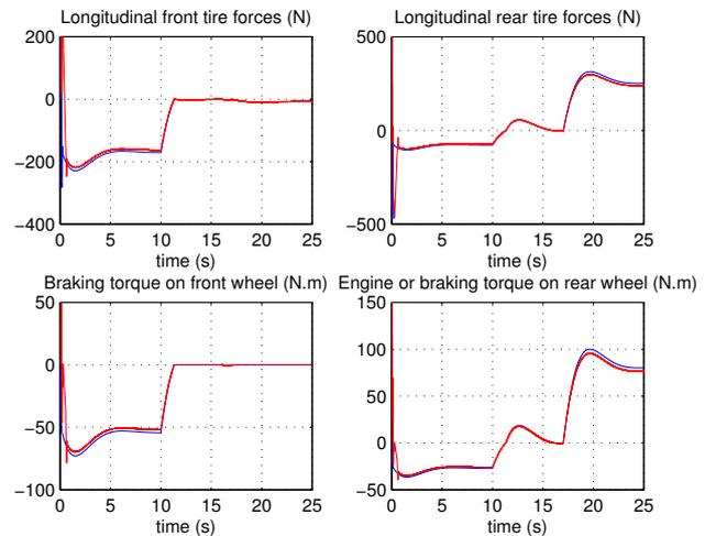
Fig. 7. **Without noises and with errors on the geometric parameters** (Top) Longitudinal front and rear forces (blue) and their estimates (red), (bottom) Front and rear engine or braking torques (blue) and their estimates (red)
