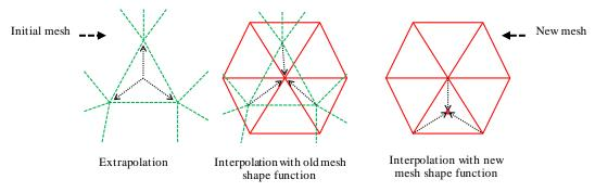
FIGURE 2. A tree-step procedure illustrating the indirect element field transfer
