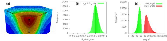
FIGURE 4. Mesh size and elements quality: (a) elements size function, (b) aspect ratio of the length of the element edges and (c) dihedral angle
