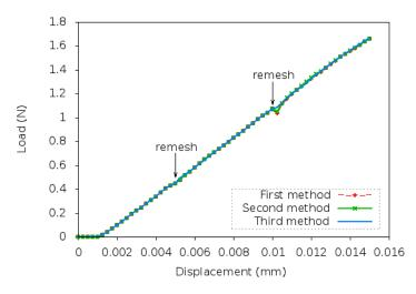
FIGURE 8. The load-displacement curves using the different adaptive strategies
