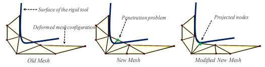
FIGURE 5. Schematic representation of the mesh correction for the contact enhancement
