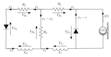
Fig. 4 Electrical circuit with resistors, inductors and ideal diodes (RLD)
