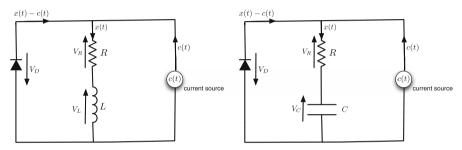
Fig. 2 Resistor-inductor-diode model (RLD, left) and resistor-capacitor-diode model (RCD, right)
