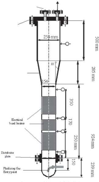
Fig. 1. Geometry of the low-scale fluidized bed
