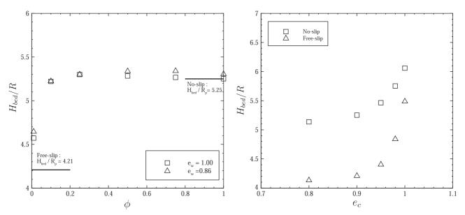
Fig. 5. Height of the bed with respect to the specularity coefficient and particle-particle restitution coefficient.
