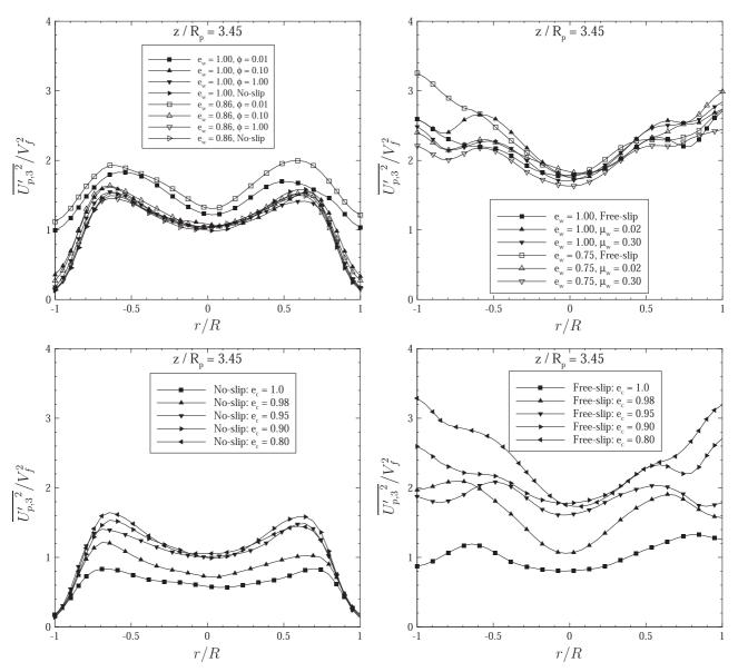
**Fig. 14.** Radial profile of the time-averaged variance of vertical solid velocity normalized by the square of fluidization velocity. Upper panels: effect of the wall boundary conditions (with the particle-particle restitution coefficient  $e_c$ =0.9), bottom panel: effect of particle-particle normal restitution coefficient, left panels: rough wall boundary conditions, right panels: smooth wall boundary conditions.
