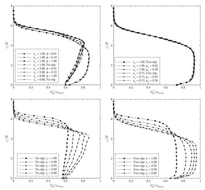
**Fig. 4.** Vertical distribution of the time-averaged solid volume fraction measured at the wall. Upper panels: effect of the wall boundary conditions (with the particle-particle restitution coefficient  $e_c$ =0.9), bottom panels: effect of particle-particle normal restitution coefficient, left panels: rough wall boundary conditions, right panels: smooth wall boundary conditions. The maximum particle solid volume fraction is  $a_{max}$ =0.64.
