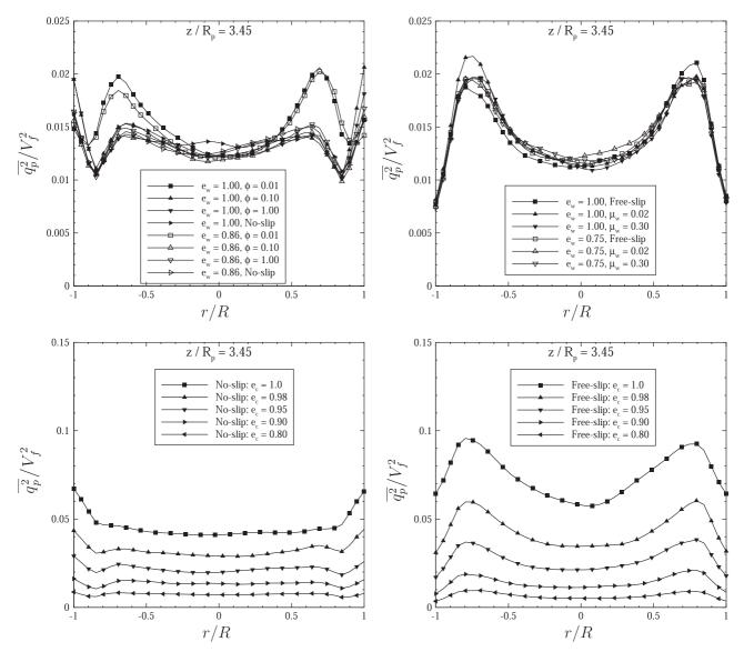
**Fig. 15.** Radial profile of the time-averaged particle kinetic energy normalized by the square of fluidization velocity. Upper panels: effect of the wall boundary conditions (with the particle-particle restitution coefficient  $e_c$ =0.9), bottom panel: effect of particle-particle normal restitution coefficient, left panels: rough wall boundary conditions, right panels: smooth wall boundary conditions.
