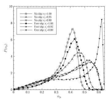
**Fig. 17.** Probability density function of the solid volume fraction in a cylinder defined such as  $-0.5 \le r/R \le 0.5$  and  $0.5 \le z/R \le 3.5$  for different values of particle-particle restitution coefficient and wall boundary type.
