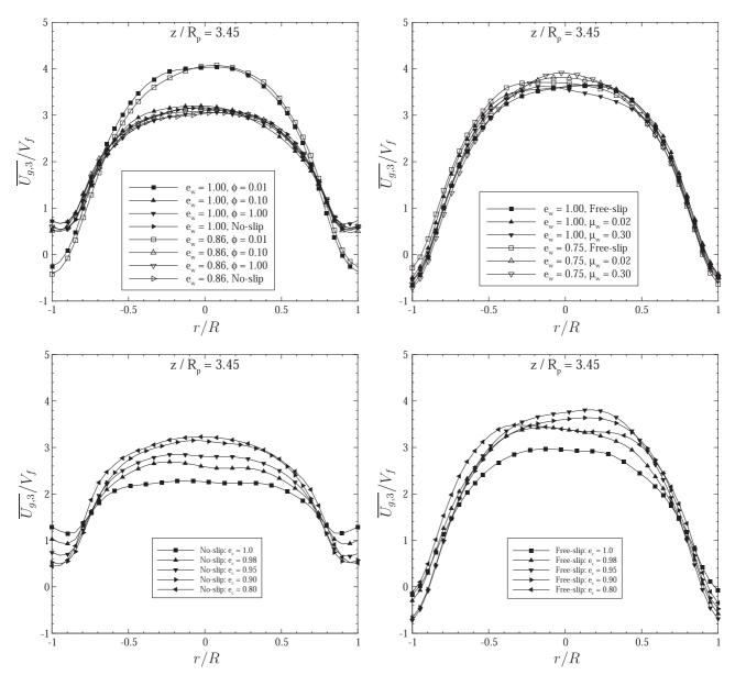
**Fig. 9.** Radial profiles of time-averaged gas vertical velocity normalized by the fluidization velocity. Upper panels: effect of the wall boundary conditions (with the particle-particle restitution coefficient, left panels: rough wall boundary conditions, right panels: smooth wall boundary conditions.
