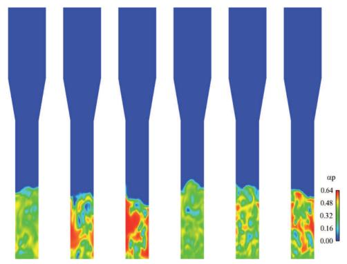
**Fig. 16.** Instantaneous solid volume fraction fields for different boundary conditions for the solid phase and different values of particle-particle restitution coefficient. From the left to the right; Free-slip and  $e_c$ =1.00, Free-slip and  $e_c$ =0.95, Free-slip and  $e_c$ =0.80. No-slip and  $e_c$ =0.95, No-slip and  $e_c$ =0.80.
