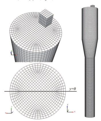
**Fig. 2.** Mesh geometry with 80245 hexahedra. Right: front view, top-left: the chimney and bottom-left: distribution plate.
