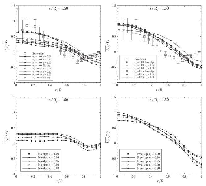
**Fig. 6.** Radial profiles of time-averaged solid vertical velocity normalized by the fluidization velocity measured at z/R = 1.50. Upper panels: effect of the wall boundary conditions (with the particle-particle restitution coefficient  $e_c = 0.9$ ), bottom panels: effect of particle-particle normal restitution coefficient, left panels: rough wall boundary conditions, right panels: smooth wall boundary conditions.
