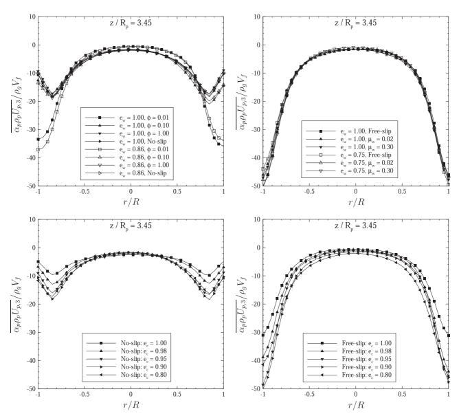
**Fig. 11.** Radial profile of the time-averaged downward solid mass flux normalized by the inlet gas mass flux. Upper panels: effect of the wall boundary conditions (with the particle-particle restitution coefficient  $e_c$ =0.9), bottom panel: effect of particle-particle normal restitution coefficient, left panels: rough wall boundary conditions, right panels: smooth wall boundary conditions.
