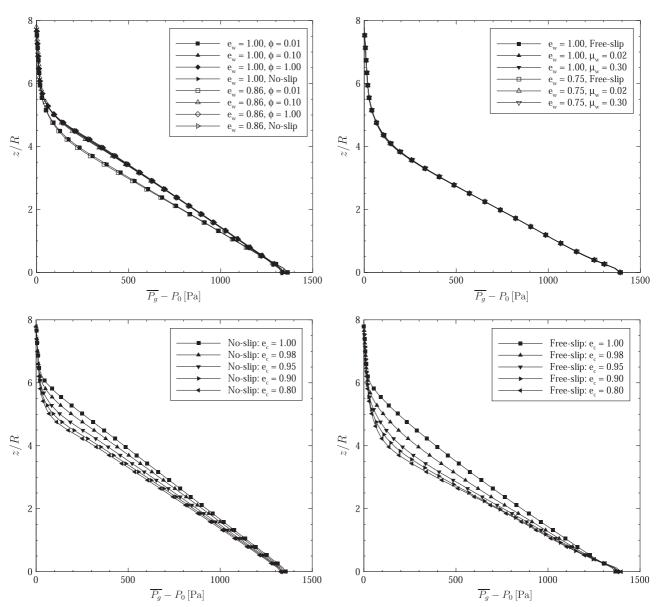
**Fig. 3.** Vertical distribution of the time-averaged gas pressure measured at the wall. Upper panels: effect of the wall boundary conditions (with the particle-particle restitution coefficient  $e_c$ =0.9), bottom panels: effect of particle-particle normal restitution coefficient, left panels: rough wall boundary conditions, right panels: smooth wall boundary conditions.
