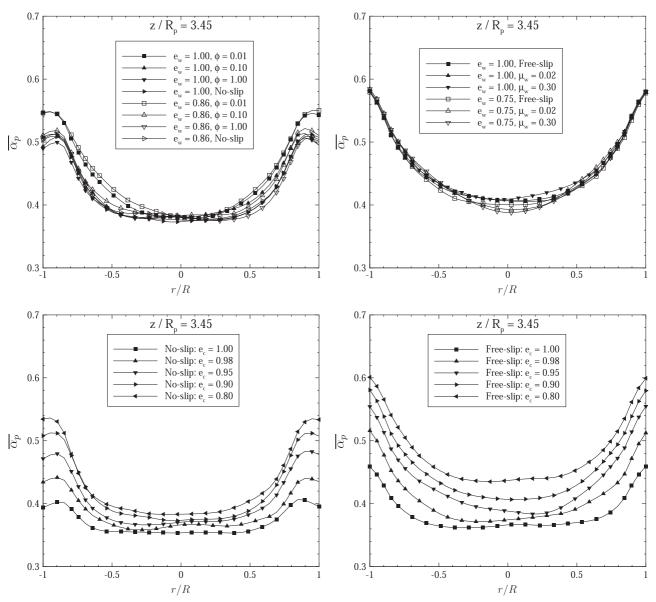
**Fig. 10.** Radial profiles of time-averaged solid volume fraction. Upper panels: effect of the wall boundary conditions (with the particle-particle restitution coefficient  $e_c$ =0.9), bottom panel: effect of particle-particle normal restitution coefficient, left panels: rough wall boundary conditions, right panels: smooth wall boundary conditions.
