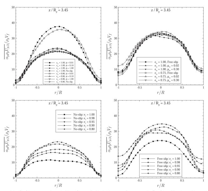
**Fig. 12.** Radial profile of the time-averaged upward solid mass flux normalized by the inlet gas mass flux. Upper panels: effect of the wall boundary conditions (with the particle-particle restitution coefficient  $e_c$ =0.9), bottom panels: effect of particle-particle normal restitution coefficient, left panels: rough wall boundary conditions, right panels: smooth wall boundary conditions.
