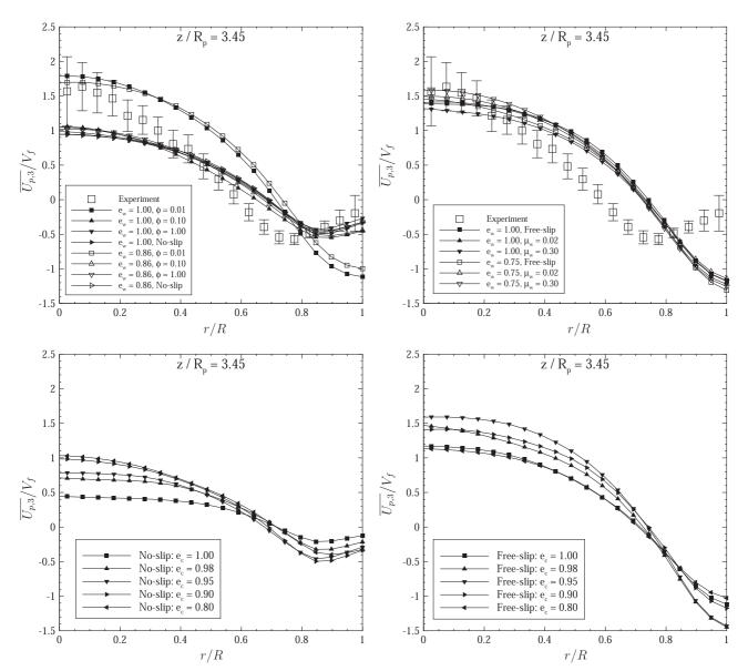
**Fig. 7.** Radial profiles of time-averaged solid vertical velocity normalized by the fluidization velocity measured at z/R = 3.45. Upper panels: effect of the wall boundary conditions (with the particle-particle restitution coefficient  $e_c = 0.9$ ), bottom panels: effect of particle-particle normal restitution coefficient, left panels: rough wall boundary conditions, right panels: smooth wall boundary conditions.
