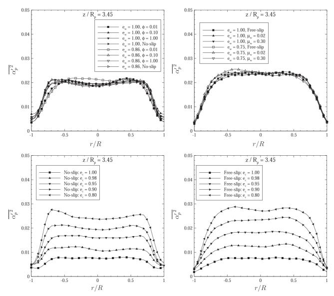
**Fig. 13.** Radial profile of the time-averaged variance of solid volume fraction. Upper panels: effect of the wall boundary conditions (with the particle-particle restitution coefficient  $e_c$ =0.9), bottom panels: effect of particle-particle normal restitution coefficient, left panels: rough wall boundary conditions, right panels: smooth wall boundary conditions
