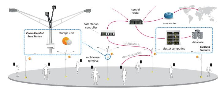
Fig. 1: An illustration of the network model. A *big data platform* is in charge of tracking/predicting users' demand, whereas *cache-enabled base stations* store the strategic contents predicted on the big data platform.
