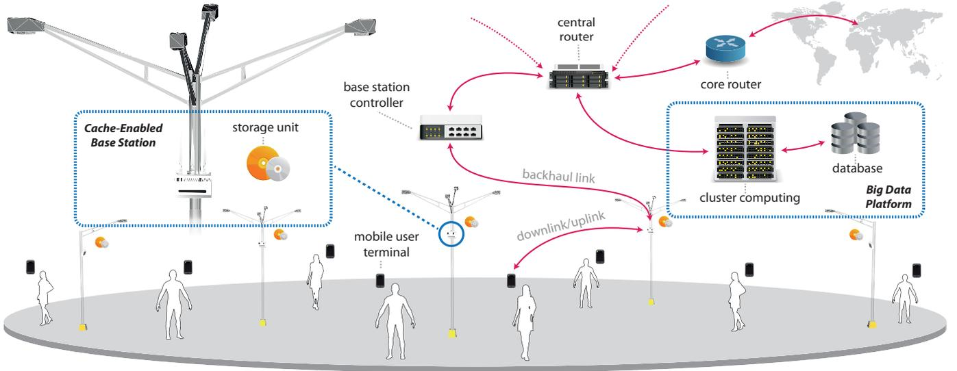
Fig. 1: An illustration of the network model. A *big data platform* is in charge of tracking/predicting users' demand, whereas *cache-enabled base stations* store the strategic contents predicted on the big data platform.
