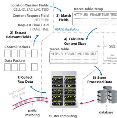
Fig. 2: An overview of the data extraction process on the big data platform.
