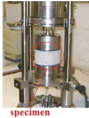
Figure 2: Experimental Set-up for the gas permeability measurement on \phi 110 \times h 50 mm specimen of concrete at 28 % aggregate volume fraction.
