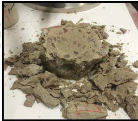
Figure 10: Damage distribution inside experimental specimen after removal
