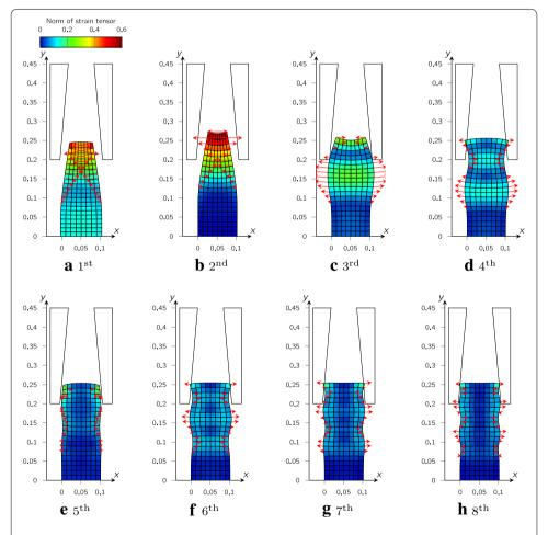
**Fig. 7** Optimal SVD spatial modes of the reference solution. *Arrows* correspond to contact force field and the *color map* refers to the norm of the strain field tensor  $\|\varepsilon\| = \sqrt{\varepsilon : \varepsilon}$
