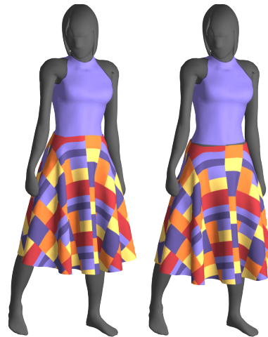
Figure 2: Naïve initialization of the rest pose by the target (left) yields sagging when statics is simulated (right), thus diverging from the target pose. In contrast, our inverse cloth design strategy allows to recover a plausible rest pose, under which the target pose matches a static configuration of the cloth simulator.
