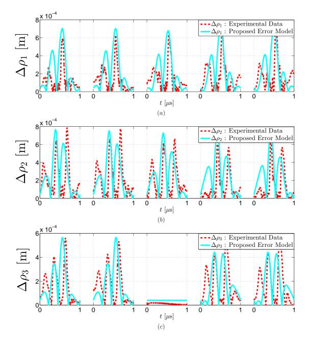
Figure 8: Joint error  $\Delta \rho_i$  and proposed error model  $\Delta \rho_i^m$  value along trajectory  $\phi_1(t)$ : [-80, -80, -140],  $\phi_2(t)$ : [-80, -80, -80],  $\phi_3(t)$ : [00, 00, 00],  $\phi_4(t)$ : [80, 80, 140],  $\phi_5(t)$ : [80, 80, 140]  $\Delta \rho_1(a_i) \Delta \rho_2(b_i) \Delta \rho_3(c_i)$ , where i = 1, 2, 3, 4, 5 which represents different trajectories
