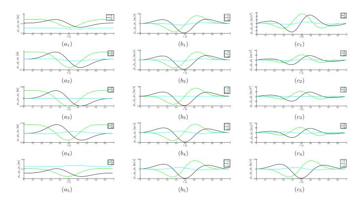
Figure 6: Joint parameters value along trajectory  $\phi_1(t)$ :  $[-80, -80, -140], \phi_2(t)$ :  $[-80, -80, -80], \phi_3(t)$ :  $[00, 00, 00], \phi_4(t)$ :  $[80, 80, 140], \phi_5(t)$ : [80, 80, 140] Joint positions  $(a_i)$  Joint velocities  $(b_i)$  Joint accelerations  $(c_i)$ , where i = 1, 2, 3, 4, 5 which represents different trajectories
