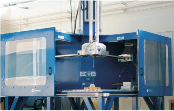
Figure 1: Semi industrial prototype of the Orthoglide 5-Axis
