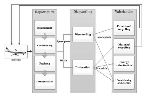
**Fig. 1.** Disassembly process representation [35].
