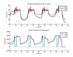
Figure 2 – Optimal command and temperature response
