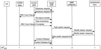
Fig. 11. Mobile relay handover procedure based on global S1 tunnel (HO)
