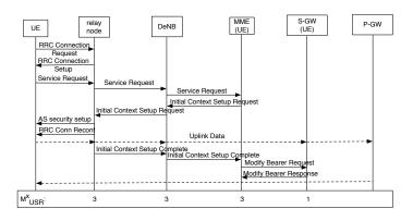
Fig. 5. UE triggered Service Request procedure (USR)
