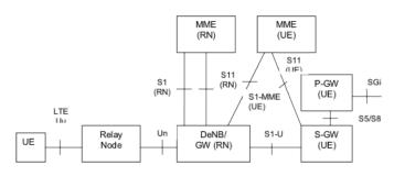
Fig. 1. Relay Architecture (source [14])
