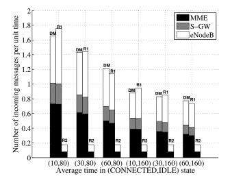
Fig. 13. Impact of the average time in ECM\_Connected state and ECM\_Idle state
