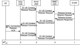
Fig. 4. Switch from CONNECTED state to IDLE state (CI)
