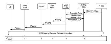
Fig. 6. Network triggered Service Request procedure (NSR)
