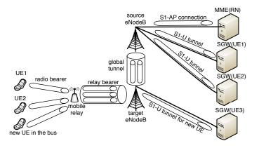
Fig. 8. The global X2 tunnel during the handover of mobile relay
