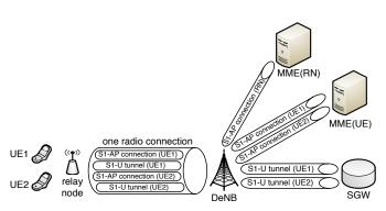
Fig. 2. Tunnels and connections with fixed relays
