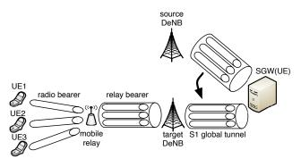
Fig. 10. The global S1 tunnel during the handover of mobile relay
