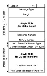
Fig. 7. Extended GTP-U header
