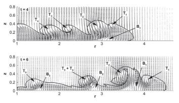
**Fig. 12.** In-plane velocity field in the vertical, y = 0, plane at t = 4 and t = 6 for Re = 10000 case. The current layout is visualized by a concentration contour of  $\phi = 0.05$ . The top (resp. bottom) vortices rotate with a counter-clockwise (resp. clockwise) direction.
