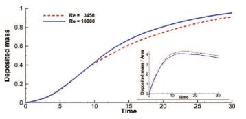
**Fig. 7.** Total mass of settled particles as a function of time for Re = 3450 and Re = 10000. Results are normalized with the initial mass of suspended particles. (Inset) Same as main figure, but results are further normalized by the horizontal area of the current and multiplied by 1000.
