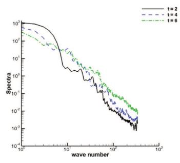
**Fig. 2.** Particle volume fraction spectra as a function of wavenumber along the x-direction for three different time instances at Re = 10000.
