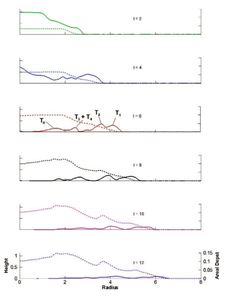
**Fig. 5.** Height (solid line) and areal deposit (dashed line) as a function of radius for different times with Re = 10000. The four peaks in the height profile at t = 6 correspond to the Kelvin–Helmholtz vortices shown in Fig. 3. The Kelvin–Helmholtz vortices at t = 4 are not as readily identifiable, perhaps because of the relatively smaller radial variations in the density profile.
