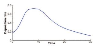
**Fig. 8.** Deposition rate versus time at the bottom wall of the domain for Re = 10000. The sedimentation rate increases from the time of release, attains a maximum value around t = 8, then monotonically diminishes up to the end of the simulation.
