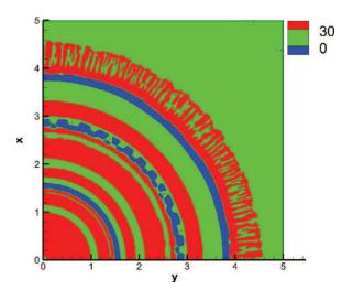
**Fig. 11.** Contours of the radial bottom shear stress for Re = 10000 in one quadrant of the computational domain at t = 6. The wall shear stress is strongly affected by the clockwise-rotating bottom vortex tubes shown in Fig. 4. Here, the wall-shear stress is multiplied by  $Re/(\rho_{c0}^*U^2)$ , where  $\rho_{c0}^*$  is the dimensional initial density of the current.
