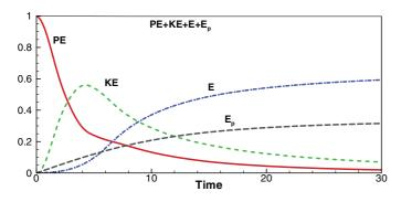
**Fig. 13.** Temporal evolution of the potential energy (PE), kinetic energy (KE), and dissipation (E and  $E_p$ ), defined in (11) and (16), respectively, of the Re = 10000 turbidity current. The sum of all four terms is shown as the thin black line.
