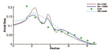
**Fig. 10.** Final areal density of deposit from simulation, experiment, and theoretical model. The experiments and theoretical model results are extracted from Bonnecaze et al. [3].
