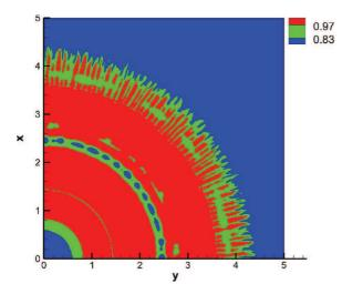
**Fig. 9.** Contours of concentration at the bottom wall for Re = 10000 in one quadrant of the computational domain at t = 6. The large scale vortex tubes transport low concentration fluid (particle-laden fluid mixed with the ambient) from the top of the current towards the bottom wall resulting in a local minimum around the radial distance r = 2.5.
