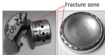
Fig. 1. Example of S360 steel application: the lid of gas generator of airbag
