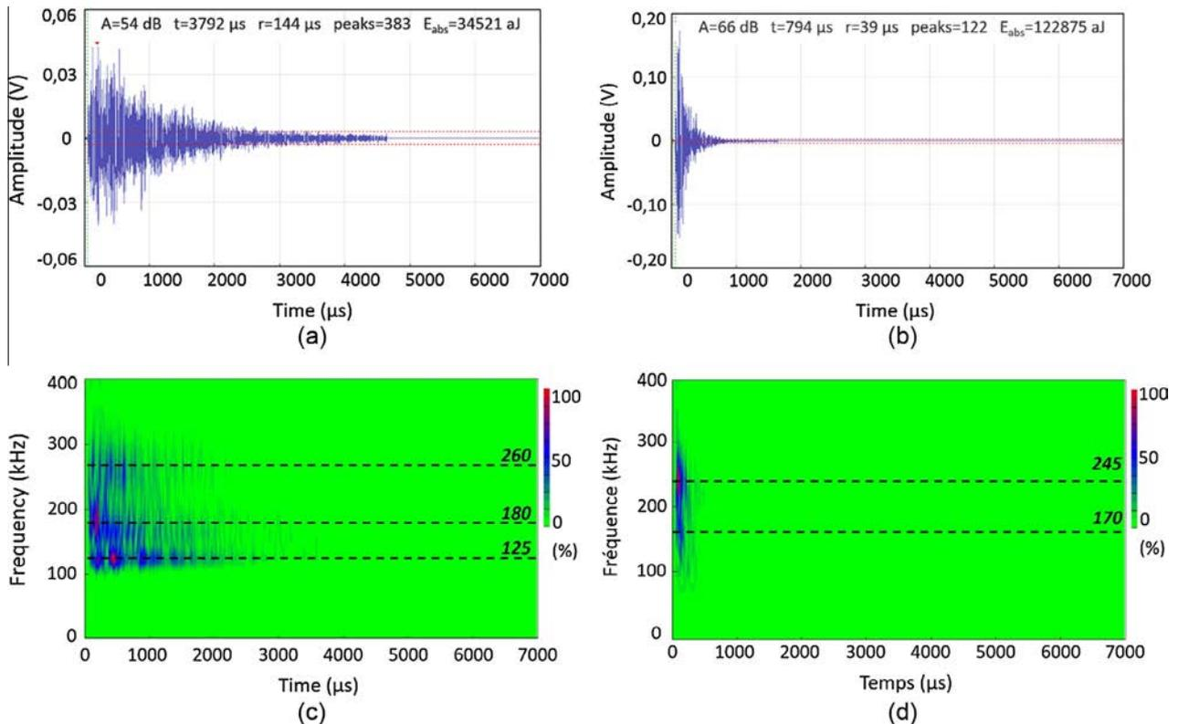
**Fig. 10.** Acoustic burst signals recorded by the AE sensor located on (a) the upper punch of the compression system, (b) on the compact, during the diametral compression test. Associated time–frequency analysis (c and d).
