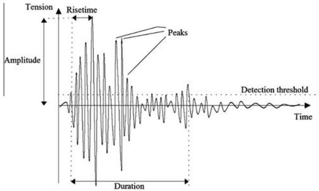
Fig. 5. Parameters of the acoustic burst signal.
