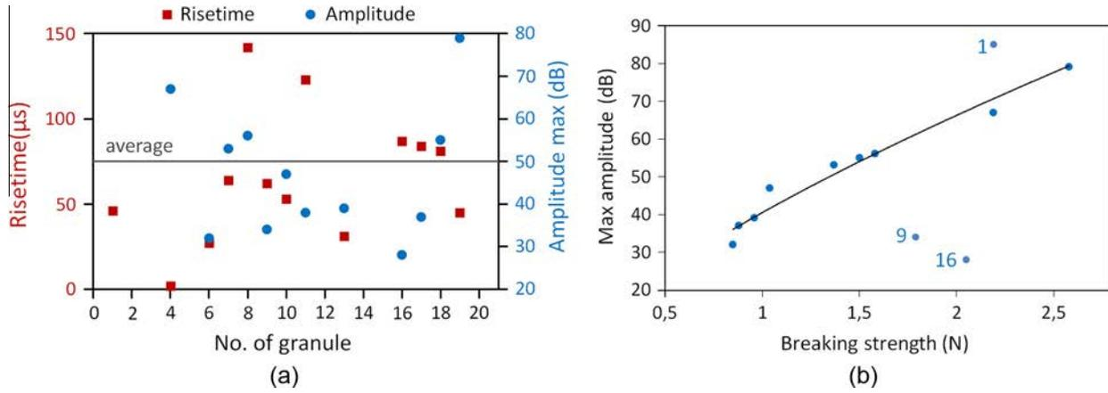
**Fig. 8.** (a) Dispersion of the burst signal parameters (rise time and maximum amplitude) for a batch of unconsolidated  $\text{UO}_2$  granules. (b) Variation of the maximum amplitude of the burst signals as a function of the breaking strength of the  $\text{UO}_2$  granules.
