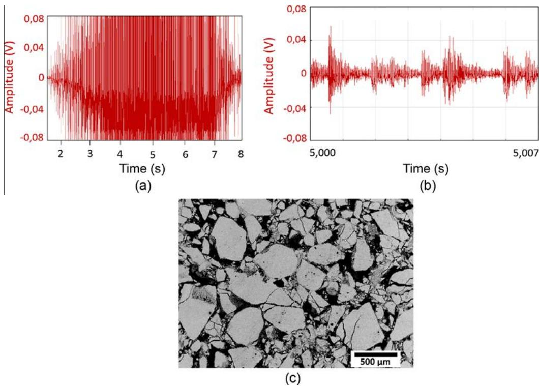
**Fig. 13.** (a) Focus on the acoustic emission, recorded between 1.6 and 8 s (Zone 2 in Fig. 11), during the compaction of a bed of brittle granules of UO<sub>2</sub>. The applied stress ranges from 0.1 to 180 MPa. (b) Focus on the burst signals recorded in the vicinity of time  $t = 5$  s. (c) SEM observations of UO<sub>2</sub> granules compacted at 5 MPa.
