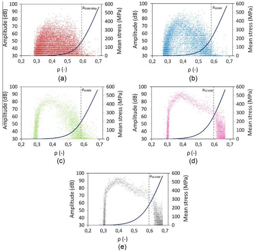
**Fig. 18.** Variation of the maximum burst amplitudes as a function of the granule bed density and the applied mean stress for five batches of  $UO_2$  granules with the 45–160  $\mu m$  size distribution and different properties of consolidation, compacted up to 600 MPa. (a) Unconsolidated granules. Thermally-consolidated granules at (b) 600 °C, (c) 800 °C, (d) 1000 °C, and (e) 1100 °C.
