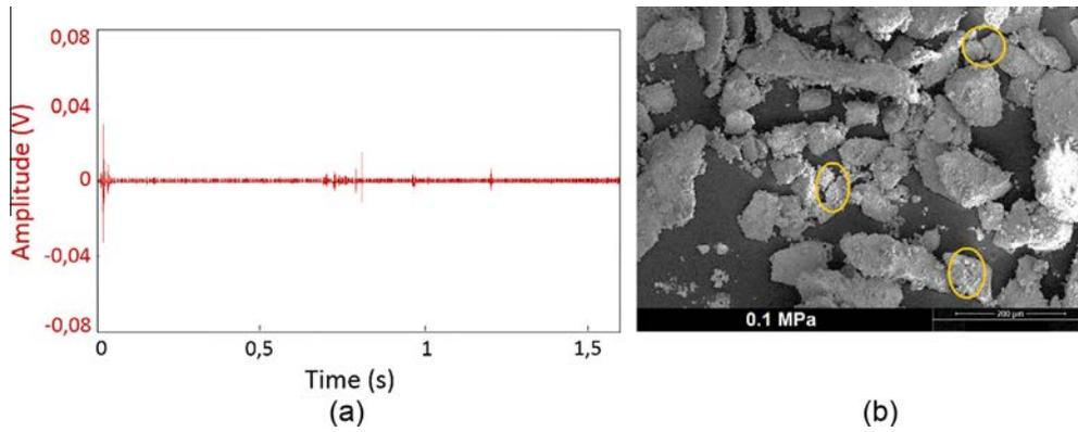
**Fig. 12.** (a) Focus on the acoustic emission, recorded between 0 and 1.6 s (Zone 1 in Fig. 11), during the compaction of a bed of brittle granules of UO<sub>2</sub>. The applied stress ranges from 0 to 0.1 MPa. (b) SEM observations of UO<sub>2</sub> granules compacted at 0.1 MPa, emphasizing granule fragmentation.
