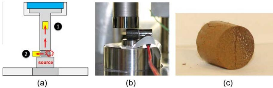
**Fig. 9.** (a) Sketch of the diametral compression test (Brazilian test) of a compact and the location of the AE sensor (in yellow). (b) Focus on the AE sensor located on the compact. (c) Fragmentation of a compact suffered a diametral compression. (For interpretation of the references to color in this figure legend, the reader is referred to the web version of this article.)
