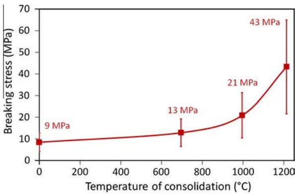
Fig. 3. Variation of the breaking stress of the  $\text{UO}_2$  granules as a function of their temperature of consolidation. The dispersion in the breaking stress at a fixed temperature results from the fact that the loading surface and the cracking surface differ from one granule to another.
