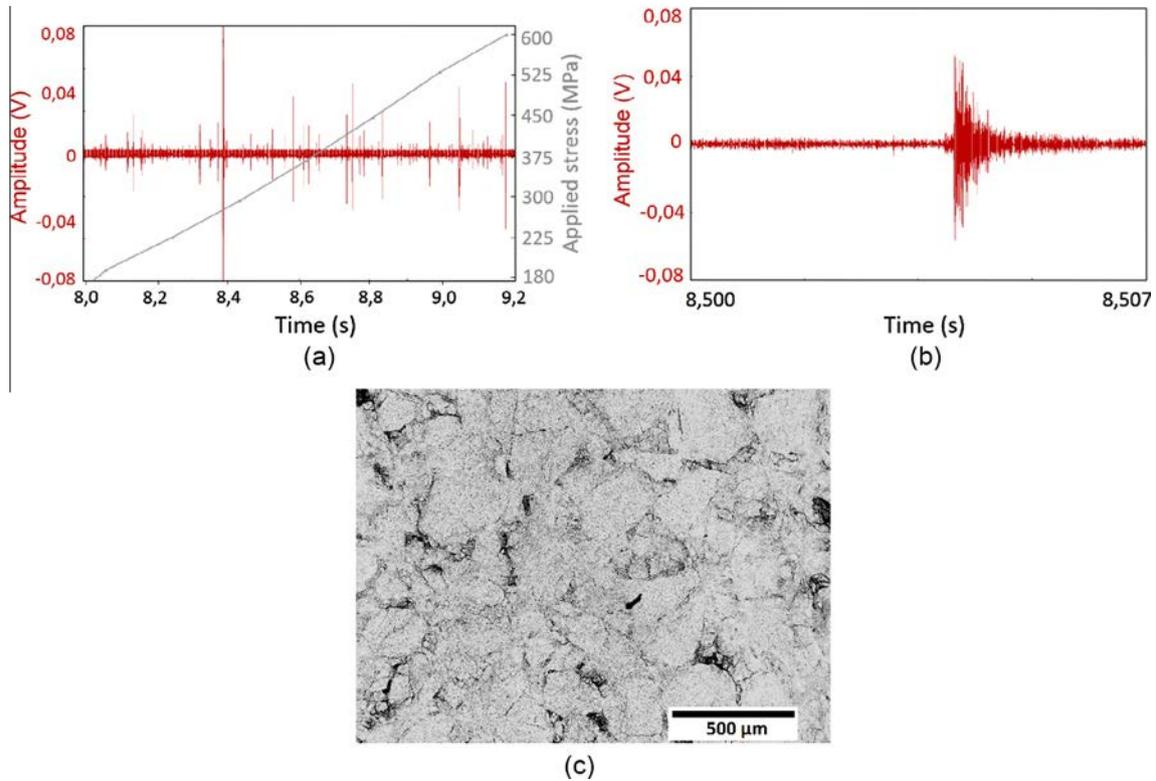
**Fig. 14.** (a) Focus on the acoustic emission, recorded above 8 s (Zone 3 in Fig. 11), during the compaction of a bed of brittle granules of  $\text{UO}_2$ . The applied stress ranges from 180 to 600 MPa. (b) Focus on the burst signals recorded in the vicinity of time  $t = 8.5$  s. (c) SEM observations of  $\text{UO}_2$  granules compacted at 300 MPa.
