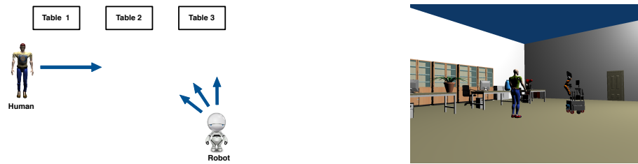
Figure 8. Experimental setup from our own experiment Lichtenthäler et al. (2012) where we measured the legibility of different navigation algorithms. The robot moves to one of the three tables and the human is crossing the robot's path. (Picture taken from Lichtenthäler et al. (2012)).
