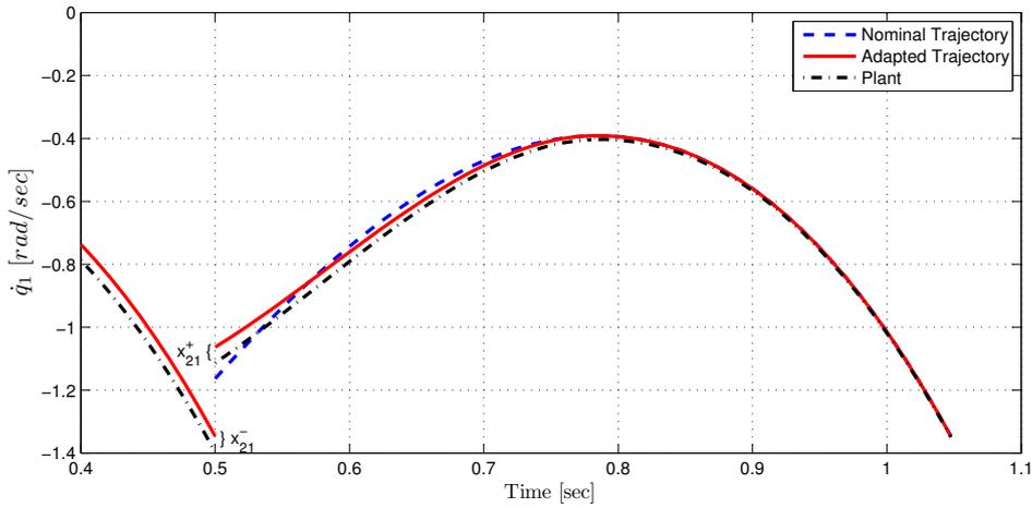
Figure 18.: Reference velocity adaptation for the first joint, with an impact at  $t^l = 0.5$ . After the impact, the initial value of the adapted velocity is such that the pre-impact  $(x_{21}(t^l-) = \dot{q}_1(t^l-) - \dot{q}_1^r(t^l-))$  and post-impact  $(x_{21}(t^l+) = \dot{q}_1(t^l+) - \dot{q}_1^r(t^l+))$  tracking errors are the same, and at the middle of the step, the adapted reference velocity reaches the nominal one.
