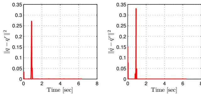
Figure 22.: Position and velocity errors  $\|\mathbf{q} - \mathbf{q}^r\|^2$  and  $\|\dot{\mathbf{q}} - \dot{\mathbf{q}}^r\|^2$  of the disturbed system. The effect of the disturbance is evident at 0.8 sec, and it is quickly attenuated by the controller.
