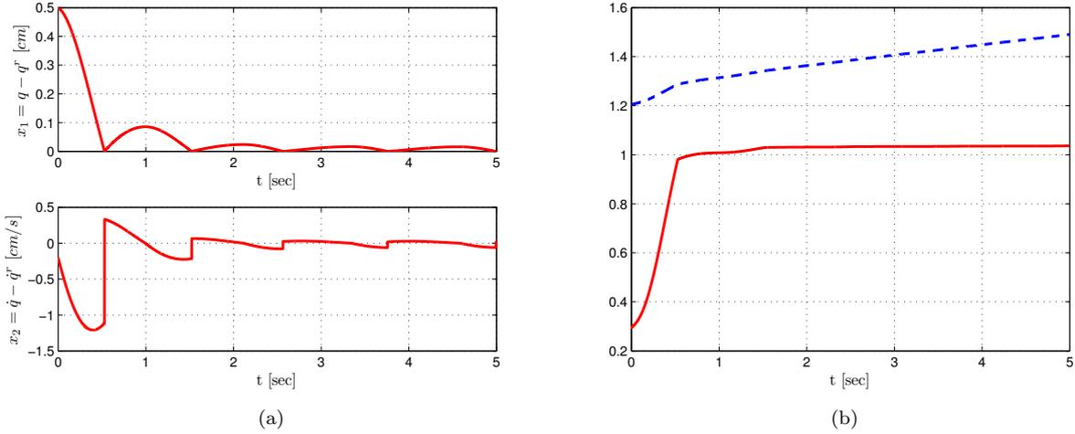
Figure 3.: Numerical results for the disturbed case of regulation problem. a) Position and velocity errors. b)  $\mathcal{L}_2$ -gain behavior for  $\gamma = 2$ :  $\|z\|_{L_2}^2 + \|z^d\|_{l_2}^2$  (solid line) versus  $\gamma^2[\|w\|_{L_2}^2 + \|w_i^d\|_{l_2}^2] + \sum_{k=0}^N \beta_k$  (dashed line).
