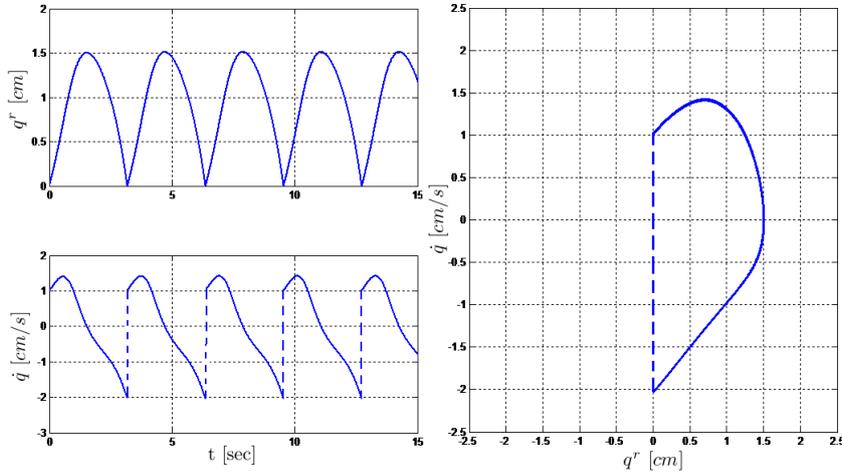
Figure 5.: Evolutions of the position  $q^r(t)$  and velocity  $\dot{q}^r(t)$  of the impact Van der Pol oscillator (??)-(??): the vertical dashed lines are for jumps in  $\dot{q}^r$  when a resetting event occurs.
