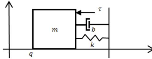
Figure 1.: Mass-Spring-Damper-Barrier (MSDB) system
