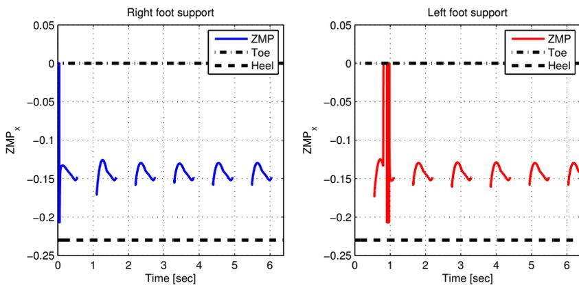
Figure 23.: Zero moment point (ZMP) location along the  $x$ -axis for each foot during its support phase. It is seen that the ZMP is always located between the toe and the heel of the supporting foot, so the walk is stable ?.
