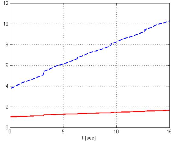
Figure 10.:  $\mathcal{L}_2$ -gain behavior without online reference model reset:  $\|z\|_{L_2}^2 + \|z^d\|_{L_2}^2$  (solid line) vs.  $\gamma^2[\|w\|_{L_2}^2 + \|w_i^d\|_{L_2}^2] + \sum_{k=0}^N \beta_k$  (dashed line) with  $\gamma = 2$ .
