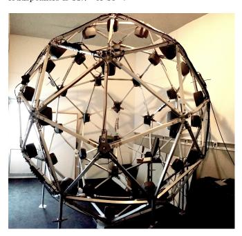
Figure 1: Picture of the spherical loudspeaker array.
