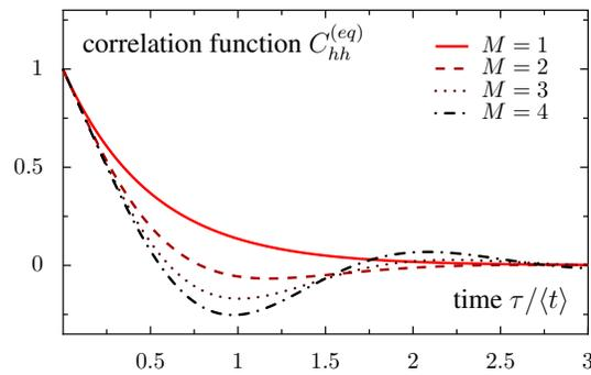
**Figure 4.** Correlation function  $C_{hh}^{(eq)}(\tau)$ , cf. Tab. 1, as a function of time  $\tau$  for the clock model. The number of ticks of the clock is denoted by  $M$ . For  $M \geq 2$ , oscillations of the correlation function are observed. The limit  $M = 1$  is special since the reversal process reduces to a Poisson process in this case. That is why correlations decay exponentially for  $M = 1$ .
