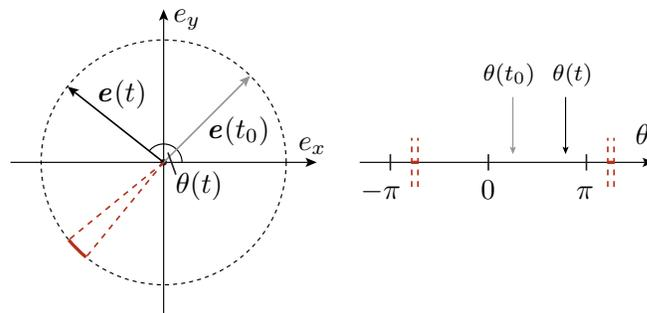
**Figure 7.** *Left:* Sketch of the temporal dynamics of  $\mathbf{e}(t)$  determining the direction of motion of a particle. The red cone indicates a region where  $\mathbf{e}(t)$  points in the opposite direction with respect to the initial direction of motion  $\mathbf{e}(t_0)$ . *Right:* The angles  $\theta$  corresponding to the vectors shown on the left.
