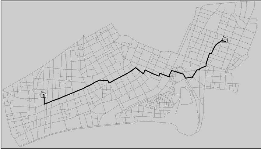
Fig. 8. Optimal itinerary minimizing environmental exposure for level pedestrian of vulnerability 1. (Distance = 3,223km; IE = 0,139)
