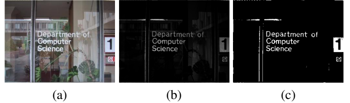
Fig. 1. GCM Results: (a) Original image, (b) Gamma Transformed Image with SGV = 5.5, (c) Output image [1].
