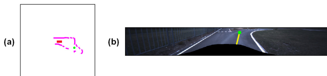
Fig. 5. Final r_{\text{obst}} and \theta_{\text{obst}} with the virtual obstacles defined by the method described in the Algorithm 1 (a) and the new image features (b), oriented to the center of the next road (green point).
