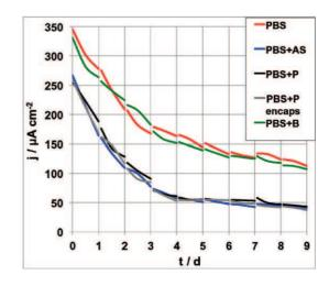
**Fig. 5.** BOx cathode performance (current density) over 9 days when polarized with constant potential of 0.3 V vs. Ag/AgCl using PBS (red), PBS + AS (blue), PBS + P (pollutants, black), PBS + P with encapsulated BOx cathode (gray) and PBS + B ("washed" bacteria, green) as electrolyte. Only one replicate is shown in the figure.
