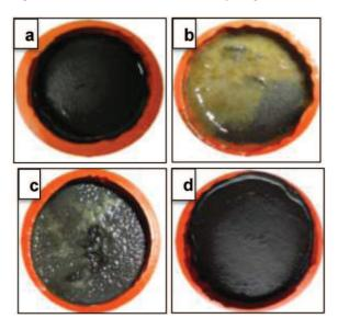
**Fig. 6.** Images of the cathodes after 45 days of constant operation in PBS (a) and in PBS + AS (b); and after 9 days of operation in presence of bacteria (PBS + bacteria) (c) and global pollutants (PBS + autoclaved AS) (d).
