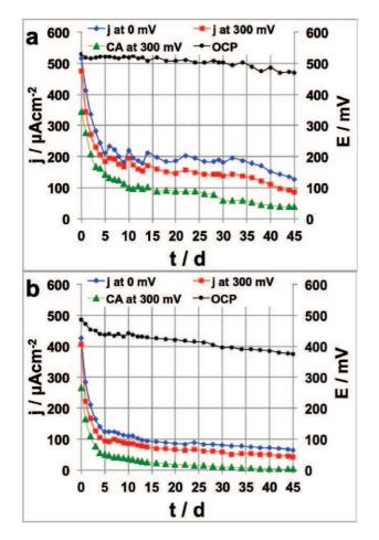
**Fig. 4.** OCP, current from the chronoamperometry at 300 mV vs. Ag/AgCl and current from the polarization curves at 300 mV and 0 mV for the BOx cathode in PBS (a) and PBS + AS (b).
