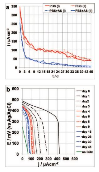
**Fig. 3.** Long-term operation of BOx cathode over 45 days when polarized with constant potential of 300 mV vs. Ag/AgCl using PBS and activated sludge (AS) as electrolyte (two replicates), with comparison to PBS-only runs (a). Representative potentiodynamic polarization curves of the BOx cathode in PBS + AS (b). Green line indicates cathode without BOx.
