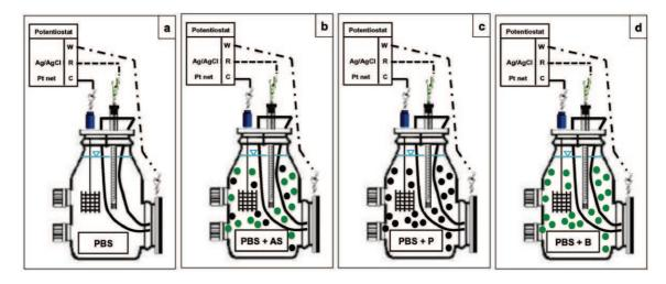
Fig. 1. Cell configuration, with the details of the four different electrolytes tested: a) PBS, b) PBS and activated sludge (50/50 mixture), c) PBS and autoclaved activated sludge (50/50 mixture) with only pollutants (P) and d) PBS and "washed" bacteria.
