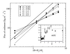
Figure 6. Flux of sediment as a function of the relative excess shear stress  $(\Theta-\Theta_c)/\Theta_c$  for different values of the sediment supply, in a log-log scale. The critical Shields number is  $\Theta_c=0.012$ . Plain lines are best fits by a power law (see Eq. 22). The bold line represents the Meyer-Peter-Müller transport law. Inset: exponent of the best fit by a power law, and its standard deviation, as a function of the sediment supply  $\sigma$ . The dotted line represents n=1.5.
