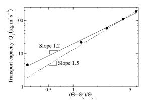
Figure 8. Saturated value  $Q_t$  of the sediment transport rate as a function of  $(\Theta - \Theta_c)/\Theta_c$ . The plain line is the best fit by a power law; the dashed line is the fit by a power law of index n = 1.5.
