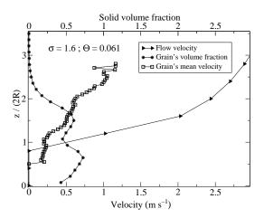
**Figure 5.** Solid volume fraction and velocity of the fluid and the pebbles as a function of height for a Shields number  $\Theta=0.061$  and a sediment supply  $\sigma=1.6$ . Two distinct layers of pebbles can be observed. The velocity of the flow and of pebbles vanishes in the bottom layer.
