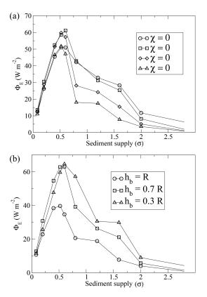
Figure 13. Flux of energy delivered to the bedrock as a function of the sediment supply for  $\Theta - \Theta_c = 0.071$ : (a) for increasing values of the roughness density  $\chi$  and (b) for different values of the roughness height.
