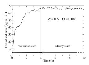
Figure 3. Flux of sediment  $q_s$  as a function of time, for a Shields number  $\Theta = 0.083$  and a sediment supply  $\sigma = 0.6$ . A transient state is observed for a few seconds before the steady state is reached.
