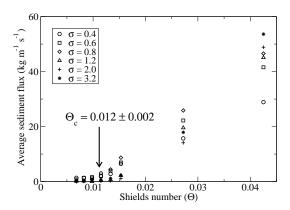
Figure 4. Average flux of sediment  $Q_{\rm S} = \langle q_{\rm S} \rangle$  as a function of the Shields number  $\Theta$  and for different values of the sediment supply  $\sigma$ .  $Q_{\rm S}$  becomes significantly larger than 0 when the Shields number exceeds  $\Theta_{\rm C} \approx 0.012$ .
