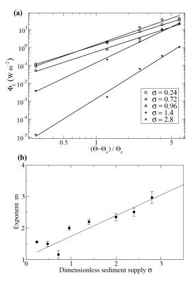
**Figure 10.** (a) Flux of energy received by the bedrock as a function of the relative excess shear stress, in a log-log scale. Plain lines are best fits of  $\Phi_{\rm E}$  with power laws (see Eq. 25). (b) Exponent  $m(\sigma)$  of the power law as a function of the dimensionless sediment supply  $\sigma$ . Data points are fitted by a linear function.
