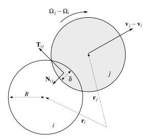
Figure 2. Two pebbles in contact, located respectively at  $r_i$  and  $r_j$ , with an overlap  $\delta = 2R - |r_i - r_j|$ .  $v_{ij}$  and  $\Omega_{ij}$  are, respectively, the translational and angular relative velocities of pebble j with respect to pebble i. Normal  $N_{ij}$  and tangential  $T_{ij}$  forces apply at the contact.
