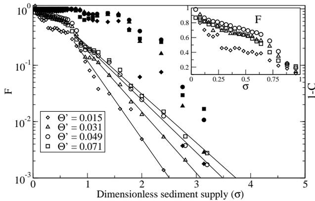
**Figure 15.** Empty symbols: cover function  $F$ , as defined by Eq. (32), plotted as a function of  $\sigma$ , in a log-linear scale. Plain lines are best fits by exponential tails for  $\sigma > 1$ . Full symbols plot  $1 - C$ , with  $C$  the static cover fraction as computed in Sect. 3.2. Inset: Zoom on the cover function for low values of  $\sigma$ , in a linear scale.
