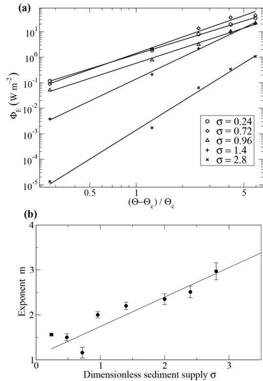
**Figure 10.** (a) Flux of energy received by the bedrock as a function of the relative excess shear stress, in a log–log scale. Plain lines are best fits of  $\Phi_E$  with power laws (see Eq. 25). (b) Exponent  $m(\sigma)$  of the power law as a function of the dimensionless sediment supply  $\sigma$ . Data points are fitted by a linear function.
