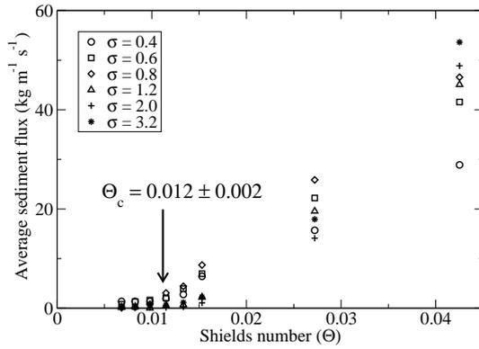
**Figure 4.** Average flux of sediment  $Q_s = \langle q_s \rangle$  as a function of the Shields number  $\Theta$  and for different values of the sediment supply  $\sigma$ .  $Q_s$  becomes significantly larger than 0 when the Shields number exceeds  $\Theta_c \approx 0.012$ .
