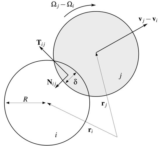
**Figure 2.** Two pebbles in contact, located respectively at  $\mathbf{r}_i$  and  $\mathbf{r}_j$ , with an overlap  $\delta = 2R - |\mathbf{r}_i - \mathbf{r}_j|$ .  $\mathbf{v}_{ij}$  and  $\Omega_{ij}$  are, respectively, the translational and angular relative velocities of pebble  $j$  with respect to pebble  $i$ . Normal  $\mathbf{N}_{ij}$  and tangential  $\mathbf{T}_{ij}$  forces apply at the contact.
