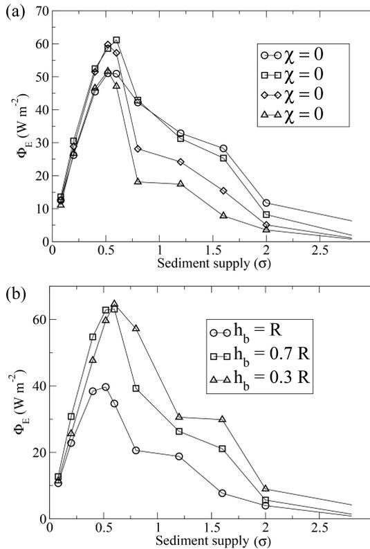
**Figure 13.** Flux of energy delivered to the bedrock as a function of the sediment supply for  $\Theta - \Theta_c = 0.071$ : (a) for increasing values of the roughness density  $\chi$  and (b) for different values of the roughness height.
