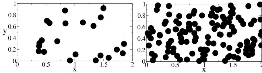
**Figure 12.** Two different cases of bedrock roughness: the positions of the glued spheres are plotted as seen from above. Left:  $\chi = 0.08$ . Right:  $\chi = 0.52$ . The flow is in the  $x$  direction, from left to right.
