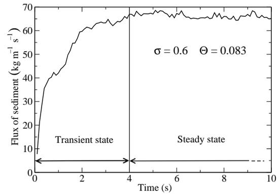
**Figure 3.** Flux of sediment  $q_s$  as a function of time, for a Shields number  $\Theta = 0.083$  and a sediment supply  $\sigma = 0.6$ . A transient state is observed for a few seconds before the steady state is reached.
