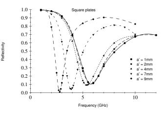
FIG. 3. Square plates in *configuration I*. Reflectivity as a function of the incident frequency, for various values of the plate's size: a' = 1, 2, 4, 7, 9mm. The period *a* is kept fixed to a = 10mm.  $\theta = 0$  and Z = 0.
