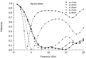
FIG. 10. Reflexion for square plates in *configuration I*. Reflectivity as a function of the incident frequency, for various values of the plate's size: a' = 1, 2, 4, 7, 9mm. The period a is kept fixed to a = 10mm.  $\theta = 0$  and Z = 0.
