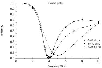
FIG. 4. Square plates in configuration I. Reflectivity as a function of the incident frequency, for various values of the plate's impedance:  $Z = 10, 30, 100\Omega/\Box$ . The period a and the plate's size a' are kept fixed a = 10mm and a' = 7mm.  $\theta = 0$ .
