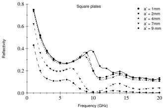
FIG. 8. Reflexion for square plates in *configuration II*. Reflectivity as a function of the incident frequency, for various values of the plate's size: a' = 1, 2, 4, 7, 9mm. The period a is kept fixed to a = 10mm.  $\theta = 0$  and Z = 0.
