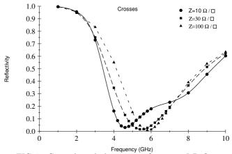
FIG. 7. Cross-shaped plates in *configuration I*. Reflectivity as a function of the incident frequency, for various values of the plate's impedance:  $Z = 10, 30, 100\Omega/\Box$ . The period *a* and the plate's size *a'* are kept fixed a = 10mm and a' = 7mm.  $\theta = 0$ .
