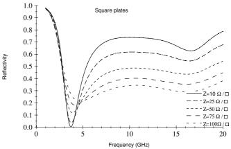
FIG. 11. Reflexion for square plates in *configura*tion *I*. Reflectivity as a function of the incident frequency, for various values of the resistive impedance *Z*:  $Z = 10, 25, 50, 75, 100\Omega/\Box$ . The period *a* is kept fixed to a = 10mm. a' = 7mm and  $\theta = 0$ .
