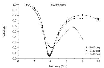
FIG. 5. Square plates in configuration I. Reflectivity as a function of the incident frequency, for various values of incidence angle:  $\theta = 10, 30, 60 \ deg$ . The period a and the plate's size a' are kept fixed a = 10mm and a' = 7mm. Z = 0.
