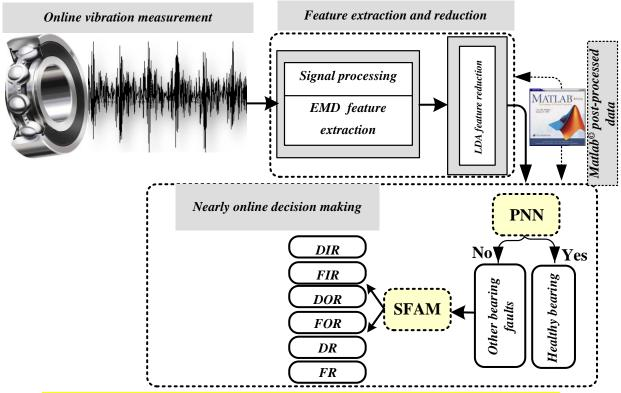
Fig. 11: General synoptic of the selected EMD-LDA-PNN-SFAM methodology.
