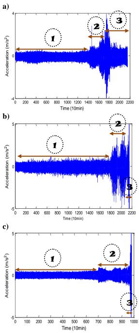
**Fig. 4:** (a) Acceleration of bearing 4 of testing 1 ending with failure roller. (b) Acceleration of bearing 3 of testing 1 ending with failure inner race. (c) Acceleration of bearing 1 of testing 2 ending with failure outer race.
