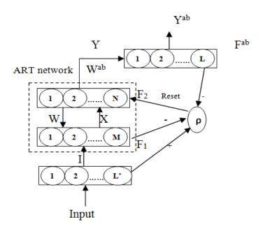
Fig. 2. SFAM neural network architecture.
