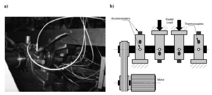
**Fig. 3:** Experimental test rig, (a) photo from the IMS center (Qiu et al., 2006), (b) simplified schematic of the test rig.
