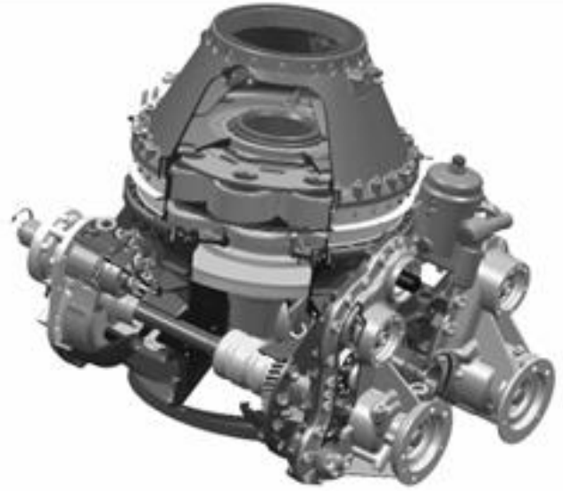
Fig. 1. Helicopter main gearbox, global view of gears.
