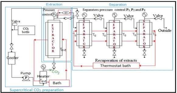
Figure 1: Diagram of dynamic extraction of carbon dioxide
