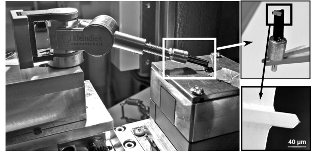
Fig. 5. Kleindiek nanomanipulator MM3A mounted inside the SEM vacuum chamber. (top-inset) End-effector fixed with a tip-less cantilever (bottom inset) SEM image of the cantilever.
