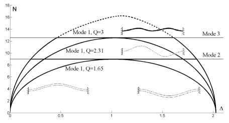
Fig. 5. Evolution of the normalized axial force N in the first kind of solution in function of Q ratio. N is constant in the second and third kinds of solution. The shape of the curved beam in the first, second and third case.
