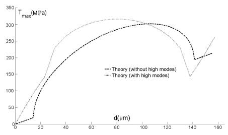
Fig. 10. Comparison between the bending maximal stress value during deflection with and without high modes of buckling.
