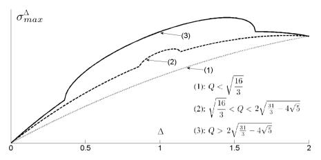
Fig. 7. Evolution of the maximal stress in the beam during deflection for different values of Q.
