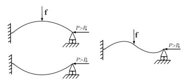
Fig. 2. Transition between the two stable positions of a buckled beam as a result of a lateral force applied in the middle of the beam.
