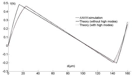
Fig. 8. Comparison of the snapping-force behavior during deflection between theory and FEM simulation.
