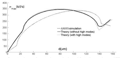
Fig. 9. Comparison between the maximal stress value during deflection between theory and FEM simulation.
