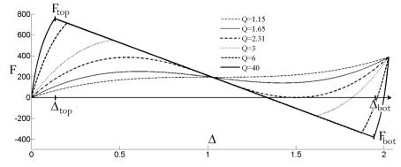
Fig. 6. Evolution of the normalized snapping force F of the pre-shaped curved beam for different Q values when mode 2 is constrained.
