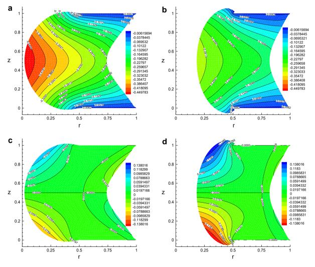
**Fig. 4.** Deformed profiles of the tube section in (*r*, *z*) space for a tube with A/B = 0.5, L/B = 1 subject to external pressure P = 2.3, with distributions of the displacement components superimposed: (a) linear *u*; (b) nonlinear *u*; (c) linear *w*; (d) nonlinear *w*.
