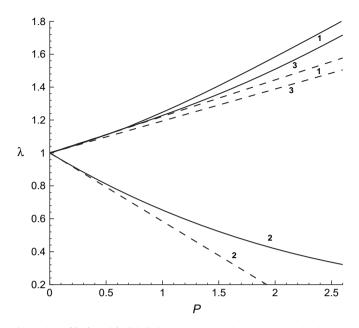
**Fig. 3.** Plots of  $\lambda_1$ ,  $\lambda_2$  and  $\lambda_3$  (labelled 1, 2, 3, respectively) versus *P* calculated at the point (*R*, *Z*) = (0.5, 0.5) for a tube with *A*/*B* = 0.5, *L*/*B* = 1: linear (dashed lines); nonlinear (solid curves).
