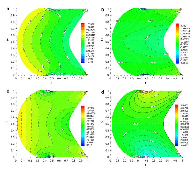
**Fig. 5.** Deformed profiles of the tube section in (r, z) space for a tube with A/B = 0.5, L/B = 1 subject to external pressure P = 2.3, with distributions of the Cauchy stress components superimposed. Linear case with positive contours (solid), negative contours (dashed): (a)  $\sigma_{11}$ , (b)  $\sigma_{22}$ , (c)  $\sigma_{33}$ , (d)  $\sigma_{13}$ .
