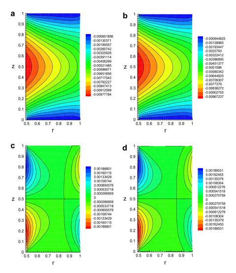
**Fig. 1.** Deformed profiles of the tube section in (r, z) space for a tube with A/B = 0.5, L/B = 1 subject to external pressure P = 0.05 with the displacement distributions u and w superimposed: (a) linear u; (b) nonlinear w; (d) nonlinear w. The plots correspond to  $R \in [0.5, 1], Z \in [0, 1]$ .
