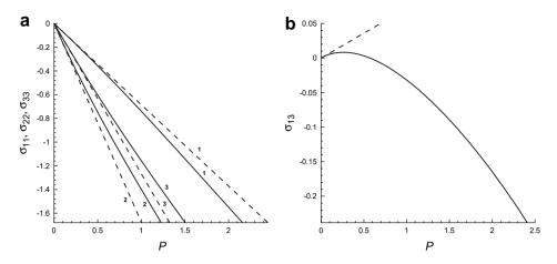
**Fig. 10.** (a) Plots of  $\sigma_{11}$ ,  $\sigma_{22}$ ,  $\sigma_{33}$  (labelled 1, 2, 3, respectively) versus *P* for a tube with A/B = 0.5, L/B = 5 at point (*R*, *Z*) = (0.75, 4.5). (b) Plots of  $\sigma_{13}$  versus *P*. Linear (dashed lines); nonlinear (solid curves).
