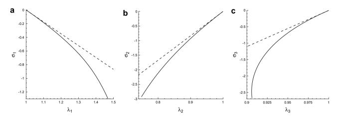
**Fig. 8.** Plots of the principal stresses versus the corresponding principal stretches for a tube with A/B = 0.5, L/B = 1 at the point (R, Z) = (0.75, 0.75): (a)  $\sigma_1$  versus  $\lambda_1$ ; (b)  $\sigma_2$  versus  $\lambda_2$ ; (c)  $\sigma_3$  versus  $\lambda_3$ . Linear results (dashed lines); nonlinear results (solid curves).
