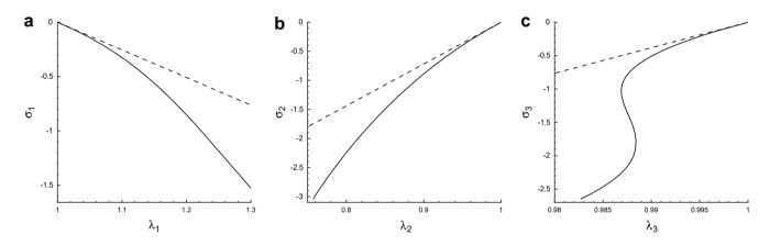
**Fig. 11**. Plots of the principal stresses versus the corresponding principal stretches for a tube with A/B = 0.5, L/B = 5, at the point (R, Z) = (0.75, 4.5): nonlinear case. (a)  $\sigma_1$  versus  $\lambda_1$ , (b)  $\sigma_2$  versus  $\lambda_2$ , (c)  $\sigma_3$  versus  $\lambda_3$ .
