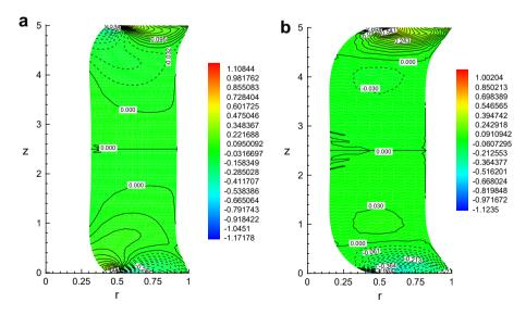
**Fig. 9.** Distributions of the shear stress  $\sigma_{13}$  for a tube with A/B = 0.5, L/B = 5 at pressure P = 1.01, superimposed on the deformed profile of tube section in (r, z) space: positive values are indicated by solid contours and negative values by dashed contours. (a) nonlinear (b) linear.
