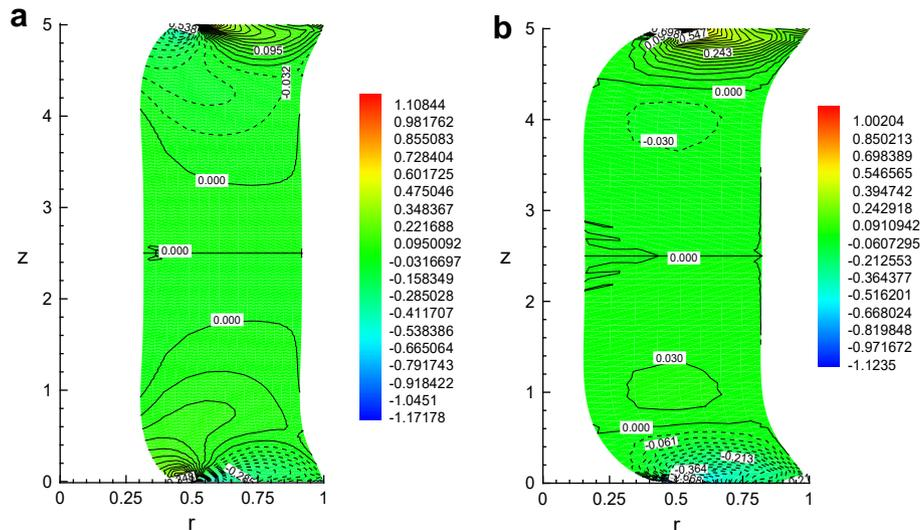
**Fig. 9.** Distributions of the shear stress  $\sigma_{13}$  for a tube with  $A/B = 0.5$ ,  $L/B = 5$  at pressure  $P = 1.01$ , superimposed on the deformed profile of tube section in  $(r, z)$  space: positive values are indicated by solid contours and negative values by dashed contours. (a) nonlinear (b) linear.
