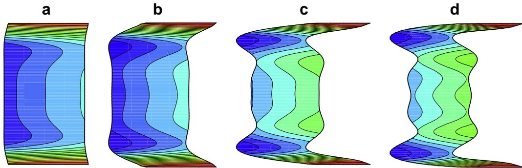
**Fig. 12.** (Not to scale) Nonlinear modes of deformation for a tube with  $A/B = 0.8$ ,  $L/B = 5$ : (a) mode-1, at  $P = 0.01$ , (b) mode-2, at  $P = 0.11$ , (c) mode-3, at  $P = 0.41$ , (d) mode-4, at  $P = 0.61$ . The contours shown are for the radial displacement  $u$  superimposed on the  $(r, z)$  deformed profile.
