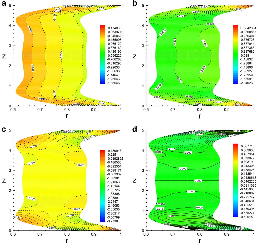
**Fig. 13.** Cauchy stress distributions for the nonlinear case for a tube with  $A/B = 0.8$ ,  $L/B = 5$  at pressure  $P = 0.22$  superimposed on the deformed tube section in  $(r, z)$  space: positive values are indicated by solid contours and negative values by dashed contours. (a)  $\sigma_{11}$ , (b)  $\sigma_{22}$ , (c)  $\sigma_{33}$ , (d)  $\sigma_{13}$ .
