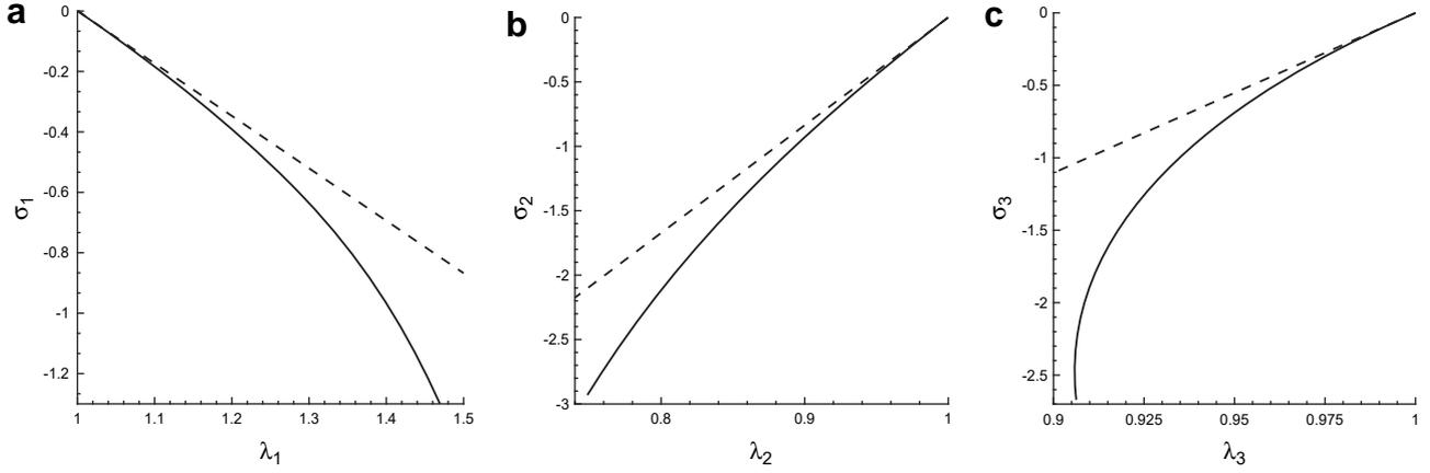
**Fig. 8.** Plots of the principal stresses versus the corresponding principal stretches for a tube with  $A/B = 0.5$ ,  $L/B = 1$  at the point  $(R, Z) = (0.75, 0.75)$ : (a)  $\sigma_1$  versus  $\lambda_1$ ; (b)  $\sigma_2$  versus  $\lambda_2$ ; (c)  $\sigma_3$  versus  $\lambda_3$ . Linear results (dashed lines); nonlinear results (solid curves).
