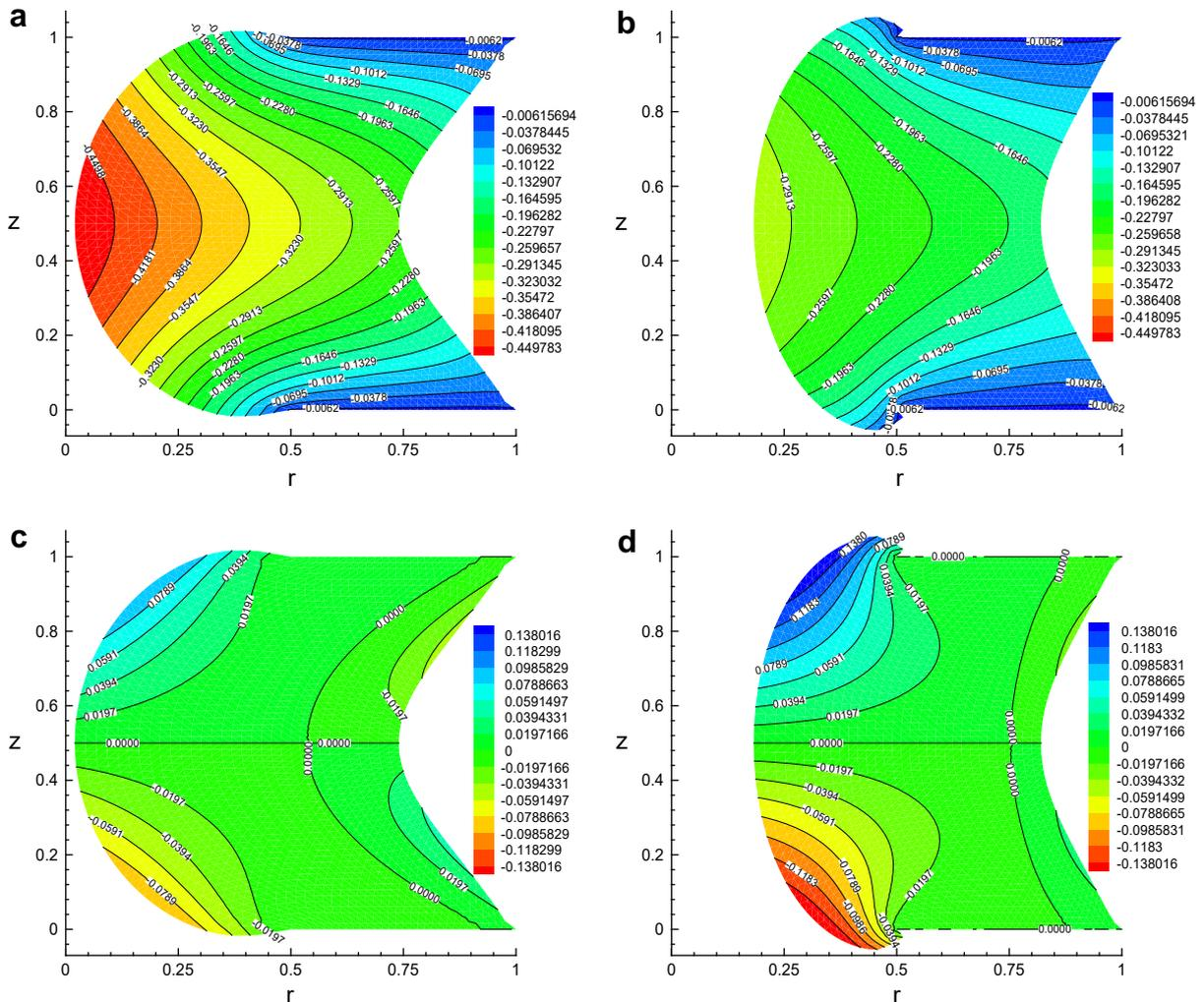
**Fig. 4.** Deformed profiles of the tube section in  $(r, z)$  space for a tube with  $A/B=0.5$ ,  $L/B=1$  subject to external pressure  $P=2.3$ , with distributions of the displacement components superimposed: (a) linear  $u$ ; (b) nonlinear  $u$ ; (c) linear  $w$ ; (d) nonlinear  $w$ .
