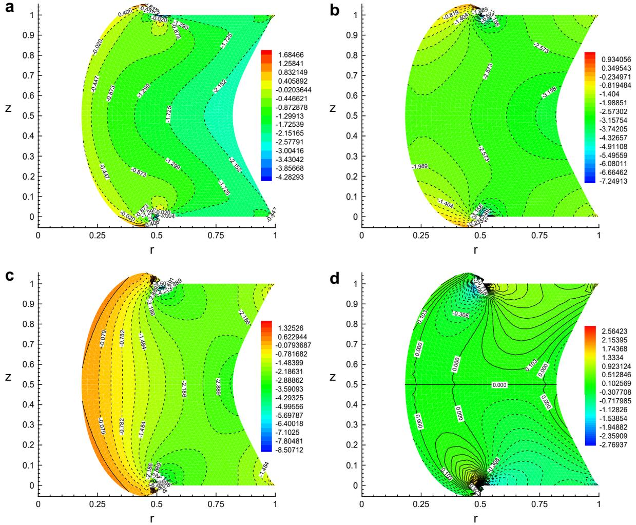
**Fig. 6.** Deformed profiles of the tube section in  $(r, z)$  space for a tube with  $A/B=0.5$ ,  $L/B=1$  subject to external pressure  $P=2.3$ , with distributions of the Cauchy stress components superimposed. Nonlinear case with positive contours (solid), negative contours (dashed): (a)  $\sigma_{11}$ , (b)  $\sigma_{22}$ , (c)  $\sigma_{33}$ , (d)  $\sigma_{13}$ .
