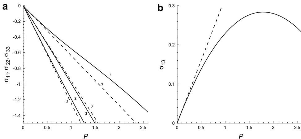
**Fig. 7.** (a) Plots of  $\sigma_{11}$ ,  $\sigma_{22}$ ,  $\sigma_{33}$  (labelled as 1, 2, 3, respectively) versus  $P$  for a tube with  $A/B=0.5$ ,  $L/B=1$  at point  $(R, Z)=(0.75, 0.75)$ . (b) Plots of  $\sigma_{13}$  versus  $P$ . Linear (dashed lines); nonlinear (solid curves).
