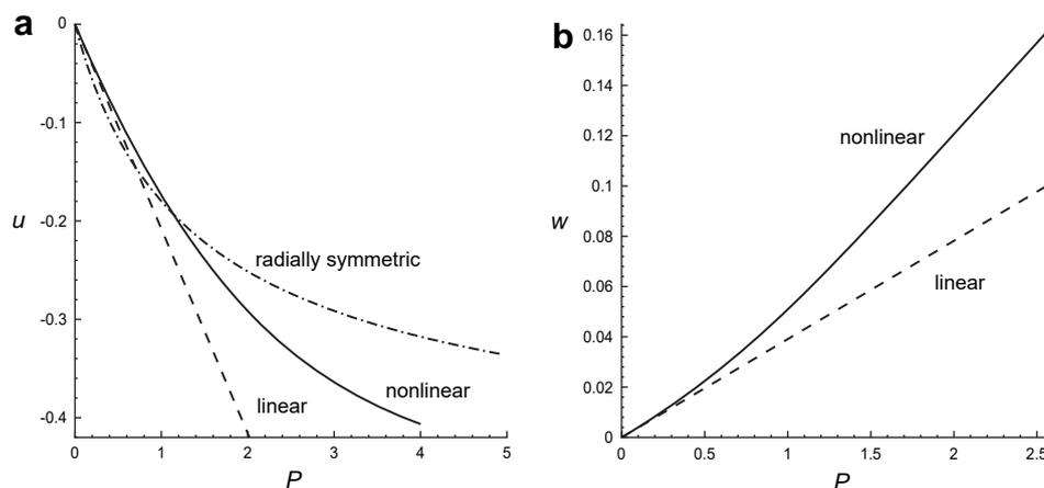
**Fig. 2.** Plots of displacement against pressure for a tube with  $A/B = 0.5$ ,  $L/B = 1$  at specific points: (a)  $u$  versus  $P$  at point  $(R, Z) = (0.5, 0.5)$ ; radially symmetric (dash-dotted curve); linear (dashed line); nonlinear (solid curve); (b)  $w$  versus  $P$  at point  $(R, Z) = (0.5, 0.75)$ ; linear (dashed line); nonlinear (solid curve).
