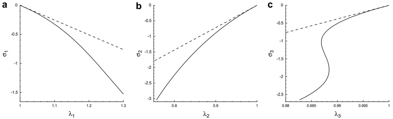
**Fig. 11.** Plots of the principal stresses versus the corresponding principal stretches for a tube with  $A/B = 0.5$ ,  $L/B = 5$ , at the point  $(R, Z) = (0.75, 4.5)$ ; nonlinear case. (a)  $\sigma_1$  versus  $\lambda_1$ , (b)  $\sigma_2$  versus  $\lambda_2$ , (c)  $\sigma_3$  versus  $\lambda_3$ .
