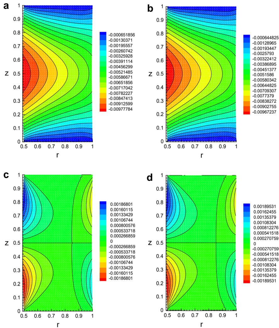
**Fig. 1.** Deformed profiles of the tube section in  $(r, z)$  space for a tube with  $A/B=0.5$ ,  $L/B=1$  subject to external pressure  $P=0.05$  with the displacement distributions  $u$  and  $w$  superimposed: (a) linear  $u$ ; (b) nonlinear  $u$ ; (c) linear  $w$ ; (d) nonlinear  $w$ . The plots correspond to  $R \in [0.5, 1]$ ,  $Z \in [0, 1]$ .
