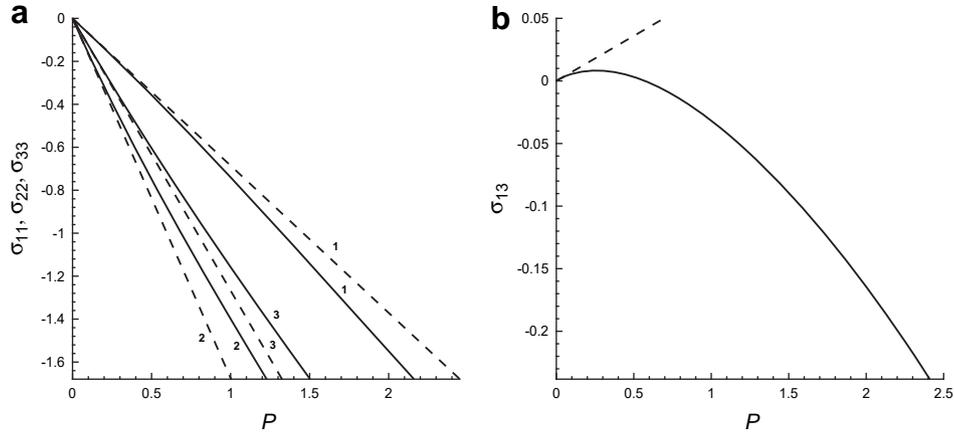
**Fig. 10.** (a) Plots of  $\sigma_{11}$ ,  $\sigma_{22}$ ,  $\sigma_{33}$  (labelled 1, 2, 3, respectively) versus  $P$  for a tube with  $A/B = 0.5$ ,  $L/B = 5$  at point  $(R, Z) = (0.75, 4.5)$ . (b) Plots of  $\sigma_{13}$  versus  $P$ . Linear (dashed lines); nonlinear (solid curves).
