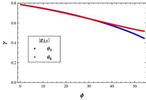
(c) Modified Bias Test. Relative rotation of the fibres in central regions vs. rotation. Second gradient energy  $g_{2,1}$ .
