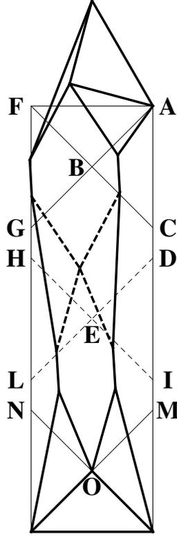
Figure 15: Modified Bias Test. Schematic of the geometry of the test.  $H/W < 4$
