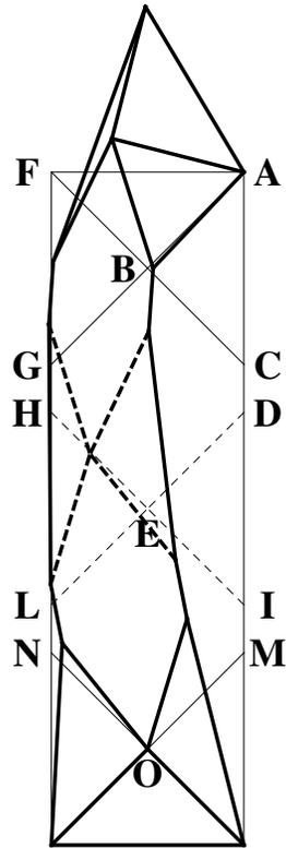
Figure 17: Modified Bias Test. Deformed shape of the specimen, quadratic second gradient energy  $g_{2,2}$ .  $H/W < 4$
