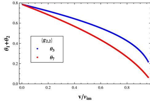
(b) BE Test. relative rotation of the fibres in central regions vs. displacement.  $H/W > 4$ . Second gradient energy  $g_{2,2}$ .
