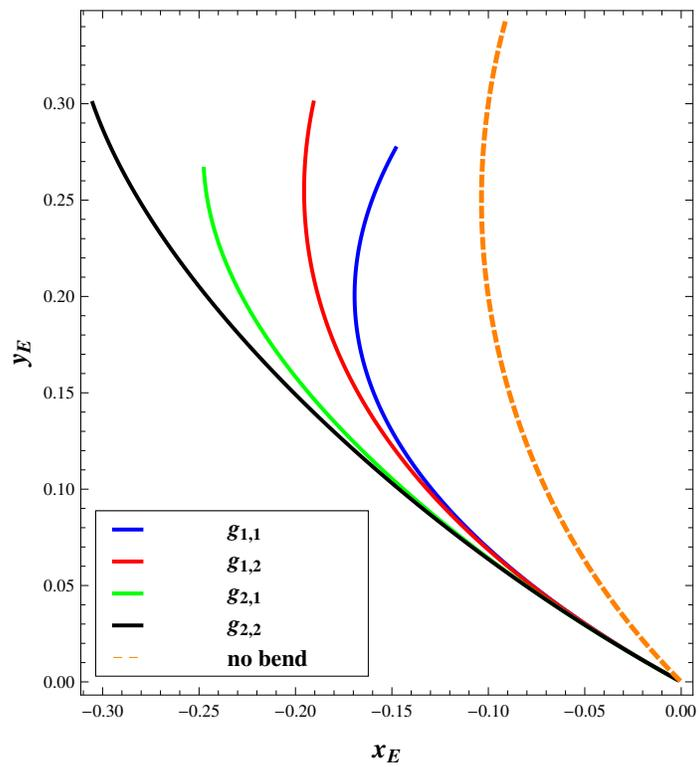
Figure 19: Modified Bias Test. Trajectory of the coordinates of the central point “E” of the specimen. All energy models. The dashed line refers to the case of a deformation without bending.
