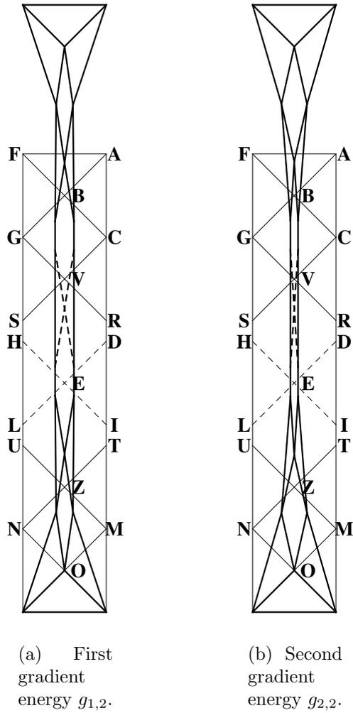
Figure 14: BE Test. Deformation of the sample.  $H/W > 4$ .
