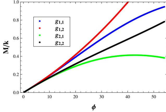
Figure 16: Modified Bias Test. Moment rotation curves obtained with four choices for the strain energy.  $H/W < 4$
