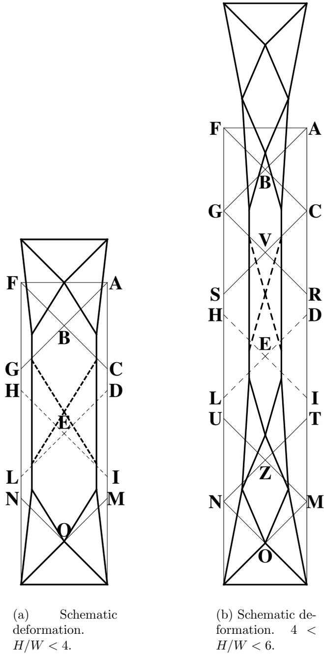
Figure 4: Bias Extension Test. Simplified kinematics.
