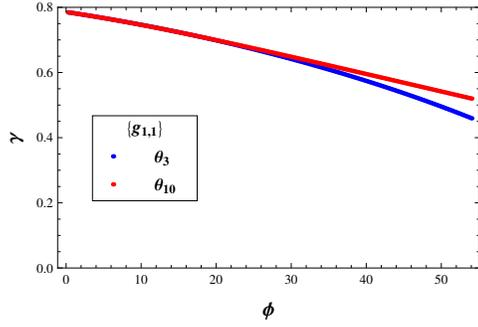
(a) Modified Bias Test. Relative rotation of the fibres in central regions vs. rotation. First gradient energy  $g_{1,1}$ .
