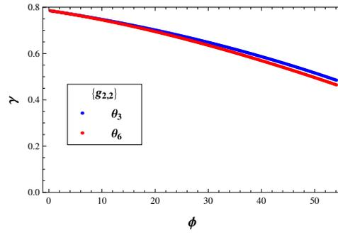
(d) Modified Bias Test. Relative rotation of the fibres in central regions vs. rotation. Second gradient energy  $g_{2,2}$ .
