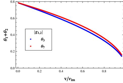
(b) BE Test. relative rotation of the fibres in central regions vs. displacement.  $H/W > 4$ . First gradient energy  $g_{1,2}$ .
