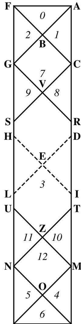
(b) Geometry of the specimen for the Bias Extension Test.  $4 < H/W < 6$ .
