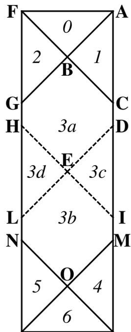
(a) Geometry of the specimen for the Bias Extension Test.  $H/W < 4$ .
