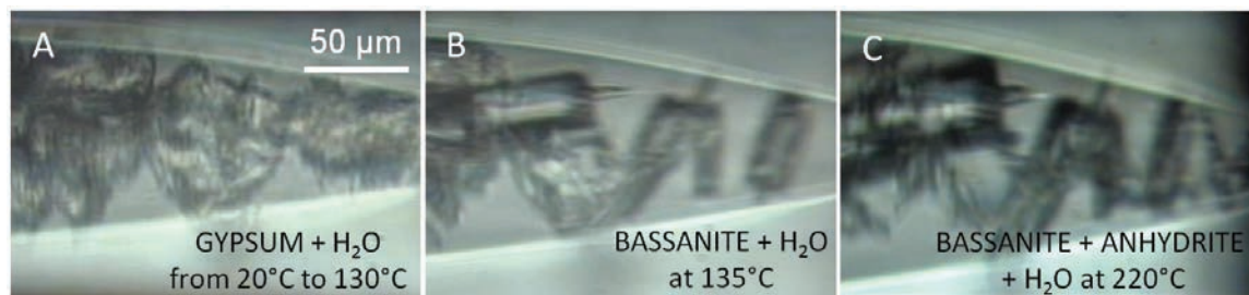
Fig. 4: Gypsum dehydration observed in a microcapillary with increasing temperature in presence of liquid water.
