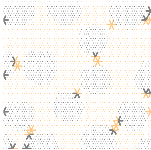
(b) Controlled elements with 5 displacement basis vectors. 28 “static” basis vectors are needed to achieve the minimal accuracy condition (32)
