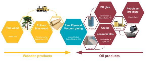
Fig. 3. Flow chart for plywood glued using a vacuum moulding technology from green veneers.
