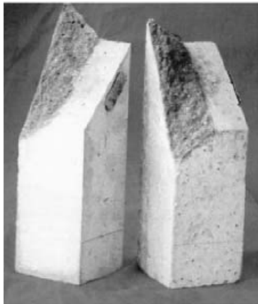
Fig. 36. Experimental crack path from [89].
