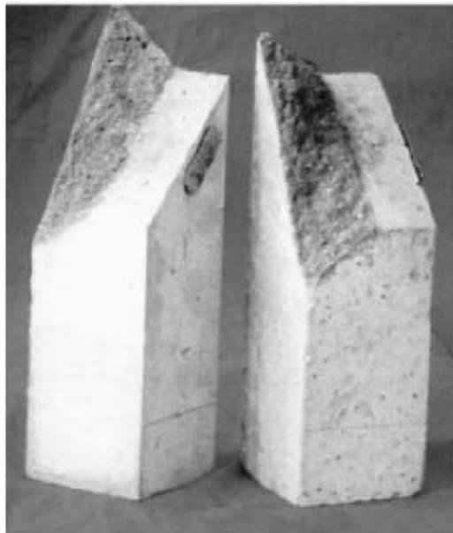
Fig. 36. Experimental crack path from [89].
