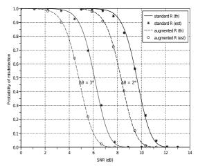
Fig.3  $P(\hat{r} < 2/r = 2)$  given by the MDL criterion associated with  $\mathbf{R}_x$  and  $\mathbf{R}_{\bar{x}}$  for two DOA separations  $\Delta\theta$  for two uncorrelated BPSK sources.
