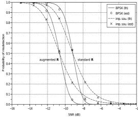
Fig.2  $P(\hat{r}=0/r=1)$  given by the MDL criterion associated with  $\mathbf{R}_x$  and  $\mathbf{R}_{\bar{x}}$  for BPSK and impulsive (p=20) distributions of the source.
