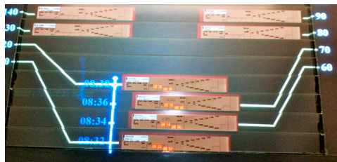
Figure 4: tangible computation of an arrival sequence: allocation within projected time slots (blue), computed stack exit times (red), strips linked to their projected stack level (white - crossing links show a misordering). This was inspired by a kind of paper ruler that is used by arrival approach controllers as rough paper that helps visualize free time slots and calculate them mentally (Fig 6).
