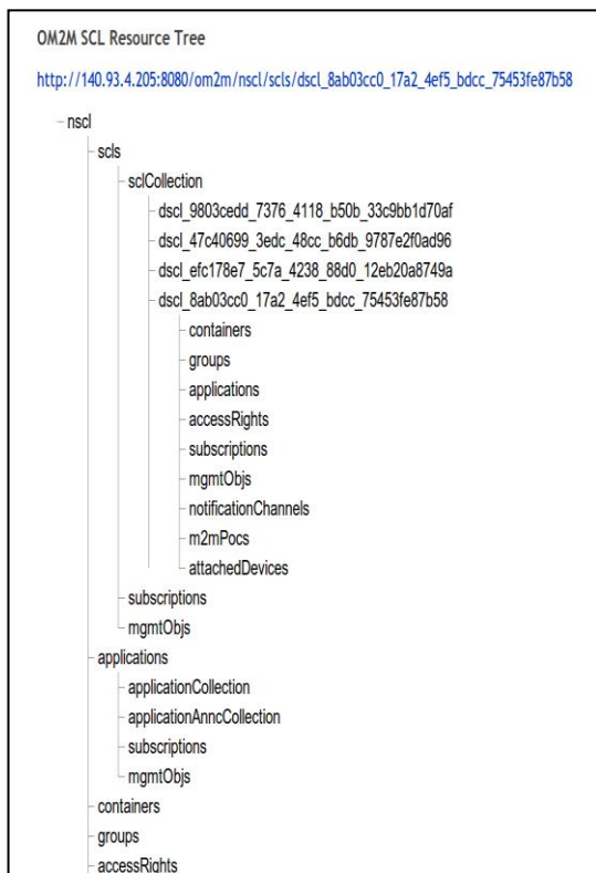
Fig 8 – Embedded solution with ETSI structure
