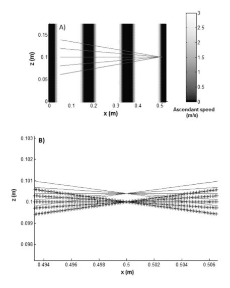
FIG 9.A) Ray propagation across ascendant flows. B) Zoom on the focusing point of the rays. Crosses: calculation of the ray path in a static medium. Line: calculation of the ray path takes into account the influence of the flow velocity.
