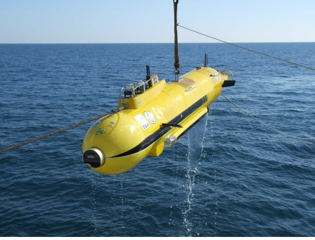
Fig. 5. Daurade : the underwater robot used for the experiment. The portside lateral sonar antenna corresponds to the one meter black segment at the bottom left of the robot
